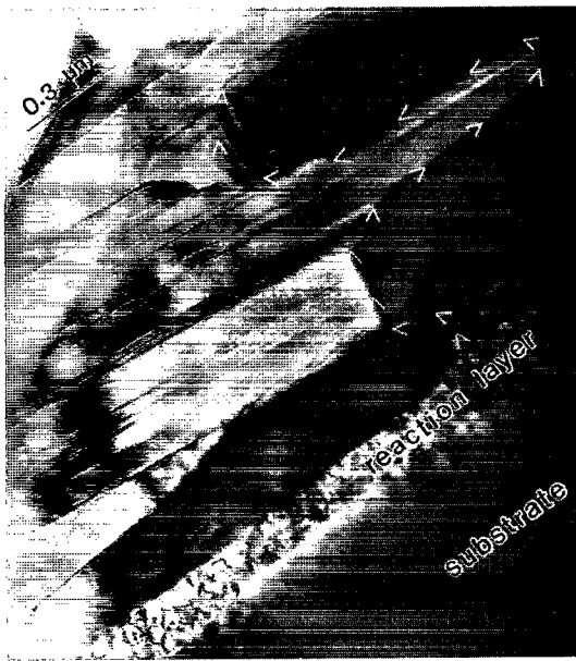
FIG. 2. TEM cross-section image showing the substrate, a thin reaction layer, and tilt (perpendicular to the substrate) and twist (parallel to the substrate) grain boundaries. As indicated by the arrows, tilt boundaries tend, in combination with short segments of twist boundary, to extend over several grains. The thin area in this view covers about half the sample thickness.
