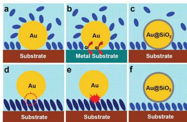
**Figure S7 | Schematic illustration of six different surface configurations for SERS or SHINERS measurements.**
