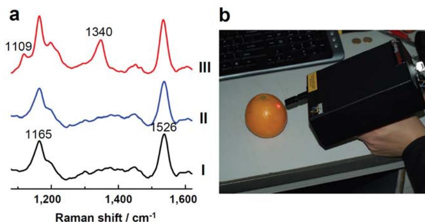
**Figure S14 | Inspecting pesticide residues on fruits with portable Raman spectrometer.** a, Normal Raman spectra on fresh citrus fruits with (I) clean pericarps and (II) contaminated by parathion. (III) SHINERS spectrum of
