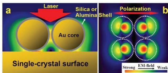
**Figure S4 | FDTD simulation of the field-enhancement.** The 3D-FDTD simulation of the optical electric field distribution of a  $2 \times 2$  array of 55 nm Au@4 nm SiO<sub>2</sub> NPs placed on a single-crystal gold surface. **a**, Side-view and **b**, Top-view of the optical electric field distribution at the gap between the particle and the surface. The shell-to-shell distance is 4 nm. The polarization of the 632.8 nm laser is indicated in **b**.
