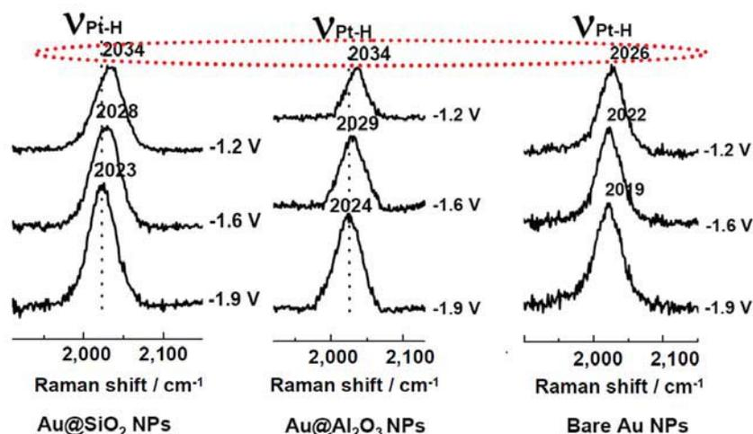
**Figure S10 | Comparison of SHIN particles with bare Au NPs on hydrogen adsorption.** SHINERS and SERS spectra of hydrogen adsorption on Pt(111) in a solution of 0.1 M NaClO<sub>4</sub> modified by (a) Au@SiO<sub>2</sub> NPs, (b) Au@Al<sub>2</sub>O<sub>3</sub> NPs and (c) bare Au NPs.
