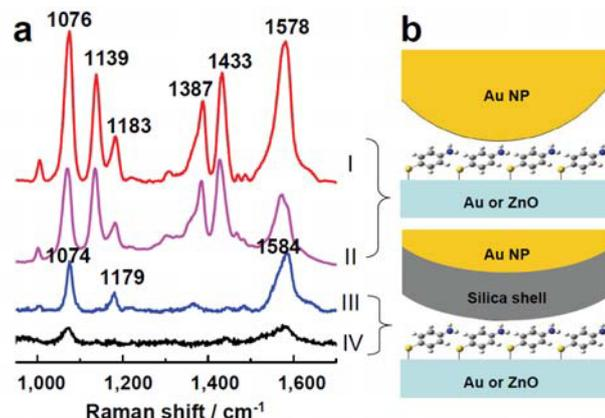
**Figure S8 | Comparison of SHIN particles with bare Au NPs on PATP adsorption.** **a**, SERS or SHINERS spectra of PATP molecules interconnected in different sandwich configurations: (I) Au/PATP/Au NPs, (II) ZnO/PATP/Au NPs, (III) Au/PATP/Au@SiO<sub>2</sub> NPs and (IV) ZnO/PATP/Au@SiO<sub>2</sub> NPs.; and the integration acquisition time, was (I) 1 s, (II) 1 s, (III) 10 s, (IV) 30s; **b**, Schematic illustration of the two different sandwich configurations.
