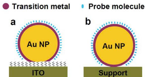
**Figure S2 | Schematic illustration of the contact mode using core-shell NPs.** (a) Coating an ultra-thin transition metal layer on Au nanoparticles dispersed electrodes by the UPD and chemical redox replacement method; (b) synthesizing Au core-transition metal shell nanoparticles by the chemical method.
