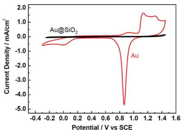
**Figure S11 | Electrochemical examination on the pinhole of the shell.** Cyclic voltammograms of 55 nm Au (red line) and 55 nm Au@4 nm SiO<sub>2</sub> (black line) NPs on glassy carbon (GC) electrodes in 0.5 M H<sub>2</sub>SO<sub>4</sub> solution. Scan rate: 0.1 V/s.
