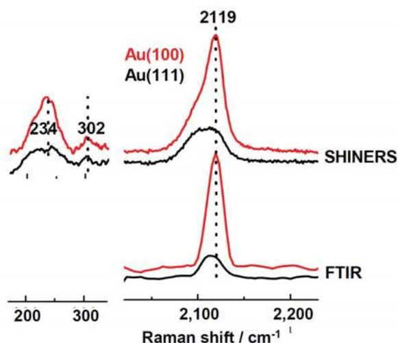
**Figure S6 | Comparison of SHINERS with FTIR spectra.** SHINERS and FTIR spectra of  $\text{SCN}^-$  adsorbed on Au(100) (red lines) and Au(111) (black lines) surfaces in the low and high wavenumber regions at 0.0 V (vs SCE). Solution: 0.01 M NaSCN and 0.1 M  $\text{NaClO}_4$ .
