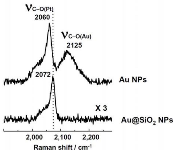
**Figure S9 | Comparison of SHIN particles with bare Au NPs on CO adsorption.** SERS and SHINERS spectra of CO adsorbed on a Pt(111) electrode surface, recorded by Au NPs (up) or Au@SiO<sub>2</sub> NPs (low) in a solution of 0.1 M HClO<sub>4</sub> saturated by CO gas.
