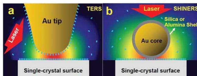
**Figure S3 | Schematic illustration of TERS and SHINERS on single-crystal surfaces in solution containing probed molecules. a, TERS as reported in literatures. b, SHINERS invented here.**
