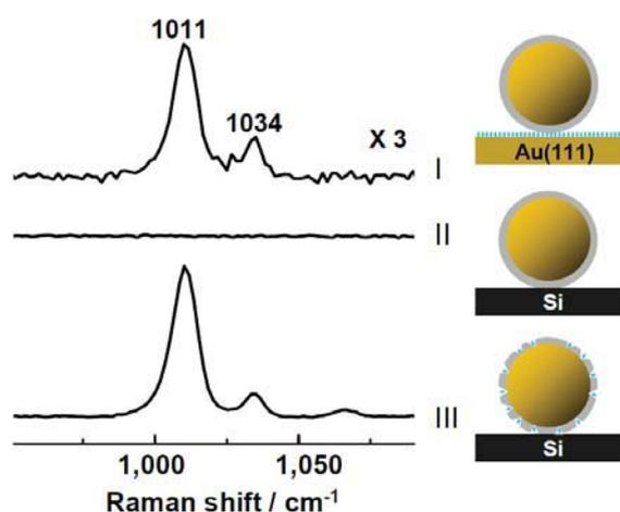
**Figure S12 | SERS examination on the pinhole of the shell.** SHINERS spectra of Py from 55 nm Au@4 nm SiO<sub>2</sub> on (I) Au(111) and (II) Si wafer, (III) 55 nm Au@1 nm SiO<sub>2</sub> NPs with pinholes on Si wafer in 0.01 M Py and 0.1 M NaClO<sub>4</sub> at -0.6 V.
