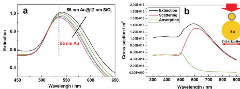
**Figure S1 | The experimental and calculated extinction spectra.** **a**, Extinction spectra of 55 nm Au@SiO<sub>2</sub> NPs with different silica shell thicknesses from about 1 nm, 2 nm, 4 nm up to 12 nm in comparison with that of bare 55 nm Au NPs. **b**, The Mie theory calculated extinction, absorption and scattering cross section of 55 nm Au@4 nm SiO<sub>2</sub> NP contacting to Au NP of 200 nm in diameter.
