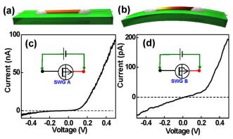
FIG. 1. (Color online) (a) A PFW lying on a polymer Kapton film substrate with two ends tightly bonded to the substrate. The leading wires connect to the measuring instrument. (b) Bending of the substrate results in the axial tensile strain and corresponding piezoelectric potential drop along the PFW. [(c) and (d)] *I-V* characteristic of SWG A and SWG B, respectively, which will be used for the studies presented in Figs. 2–4.
