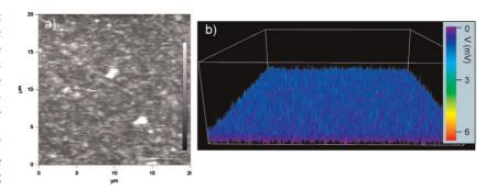
**Figure 2.** a) AFM image acquired from an array of semiconductive Si nanowires, which shows the tips of the nanowires. b) The corresponding piezoelectric potential output image across the sample measured by the AFM tip in contact mode. Within the experimental noise range, the Si nanowires produced no electricity. Transport measurement of the nanowire did show that they conducted electricity. The experimental set up and conditions were the same as in [1].
