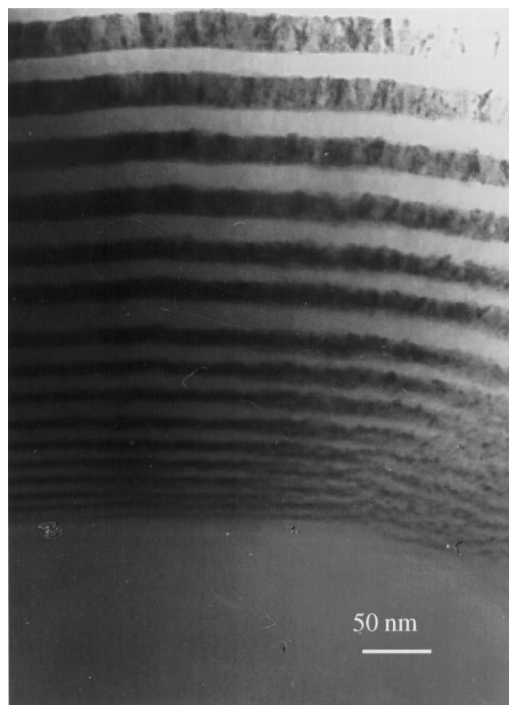
Fig. 2. A bright-field TEM cross-sectional image of the composite showing the progression of matrix layers from fiber surface.
