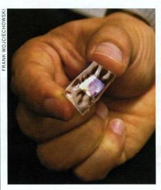
wire-based nanogenerator (*Adv. Mater.*, DOI: 10.1002/adma.200904355). Even though he has yet to test the system in humans, he says that his ZnO nanowires are biodegradable.
