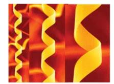
Scanning electron microscopy images of the semiconucting and piezoelectric zinc oxide nanohelix. (Courtesy: ZL Wang)
