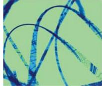
Georgia Tech's Z. L. Wang and his group discovered zinc oxide nanobelts in 2001. These nanobelts define a new group of nanomaterials for applications in nanoelectronics, nanosensors, nanoactuators, and biosensors This performance is demonstrated in the company's two-position tab, which can be mounted on the trailing edge of a helicopter rotor blade. It replaces the standard mechanical tabs that are manually adjusted between flights to balance the rotor blades and minimize vibration.
