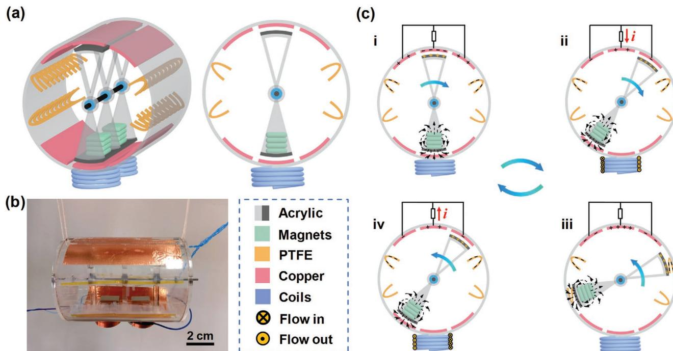
**Figure 1.** a) Schematic representation of the swing-structured triboelectric–electromagnetic hybrid nanogenerator, including the 3D structure and cross-section view. b) Photograph of the fabricated hybrid TENG/EMG device. c) Schematic illustration for the working principle of the hybrid nanogenerator.
