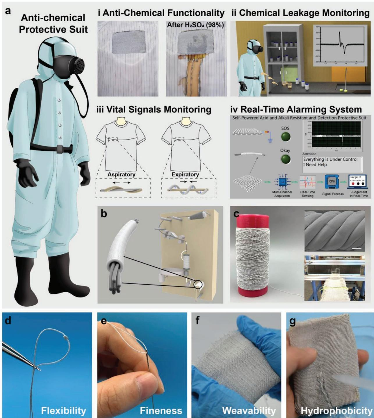
**Figure 1.** Schematic illustration of SETY, F-TENG, and intelligent anti-chemical protective suit. a) Schematic of anti-chemical protective suit, which has four functions of anti-chemical property, chemical leakage monitoring, vital signal monitoring, and real-time alarm system. b) Schematic of SETY fabricating process. c) Photograph and SEM image of SETY and F-TENG fabricating process. d,e) Images of SETY. f,g) Images of F-TENG.
