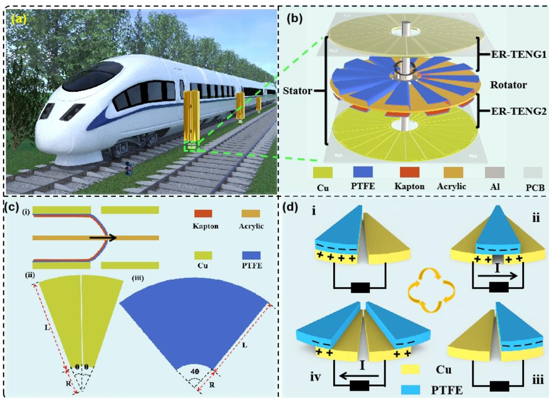
**Figure 1.** Structural design and working mechanism of ER-TENG. (a) Device configuration of double-layer ER-TENGs installed on both sides of the railway track at intervals. (b) Schematic representation of the structure of the double-layer ER-TENG. (c) A geometric structure design drawing of an ER-TENG. (d) The electricity generation principle of each TENG unit of the ER-TENG.
