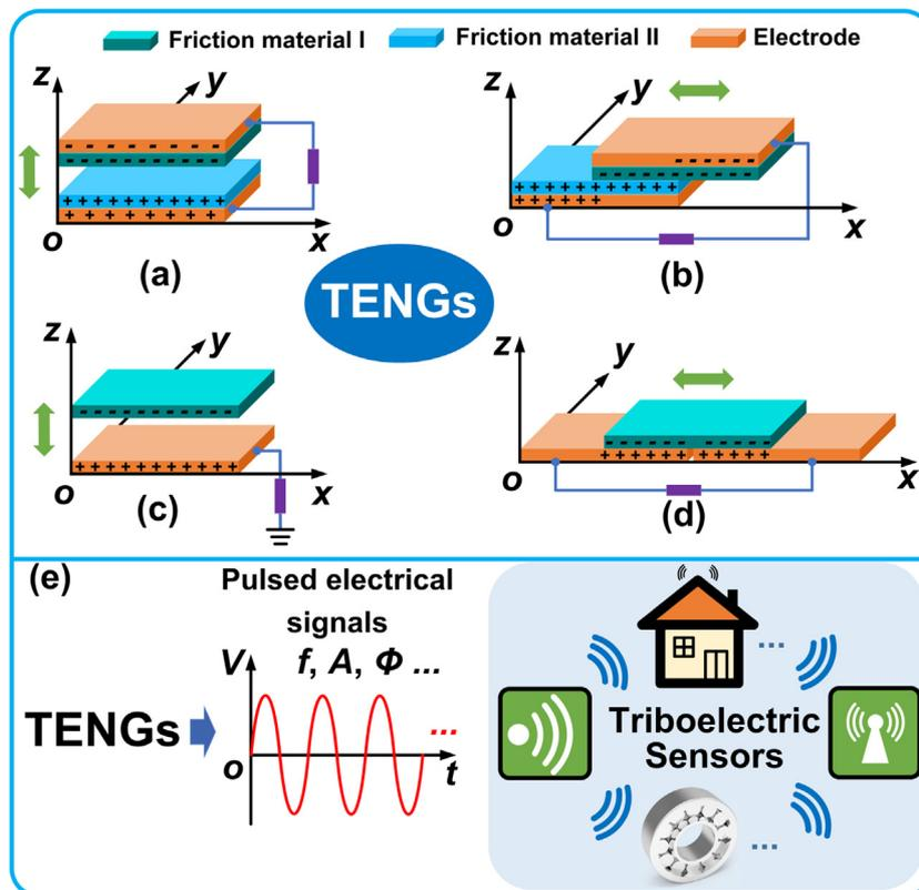
Fig. 2. The four working modes of TENGs and the physical basis of the triboelectric sensors. (a) The vertical contact-separation mode. (b) The contact-sliding mode. (c) The single-electrode mode. (d) The freestanding triboelectric-layer mode. (e) The physical basis of the triboelectric sensors.
