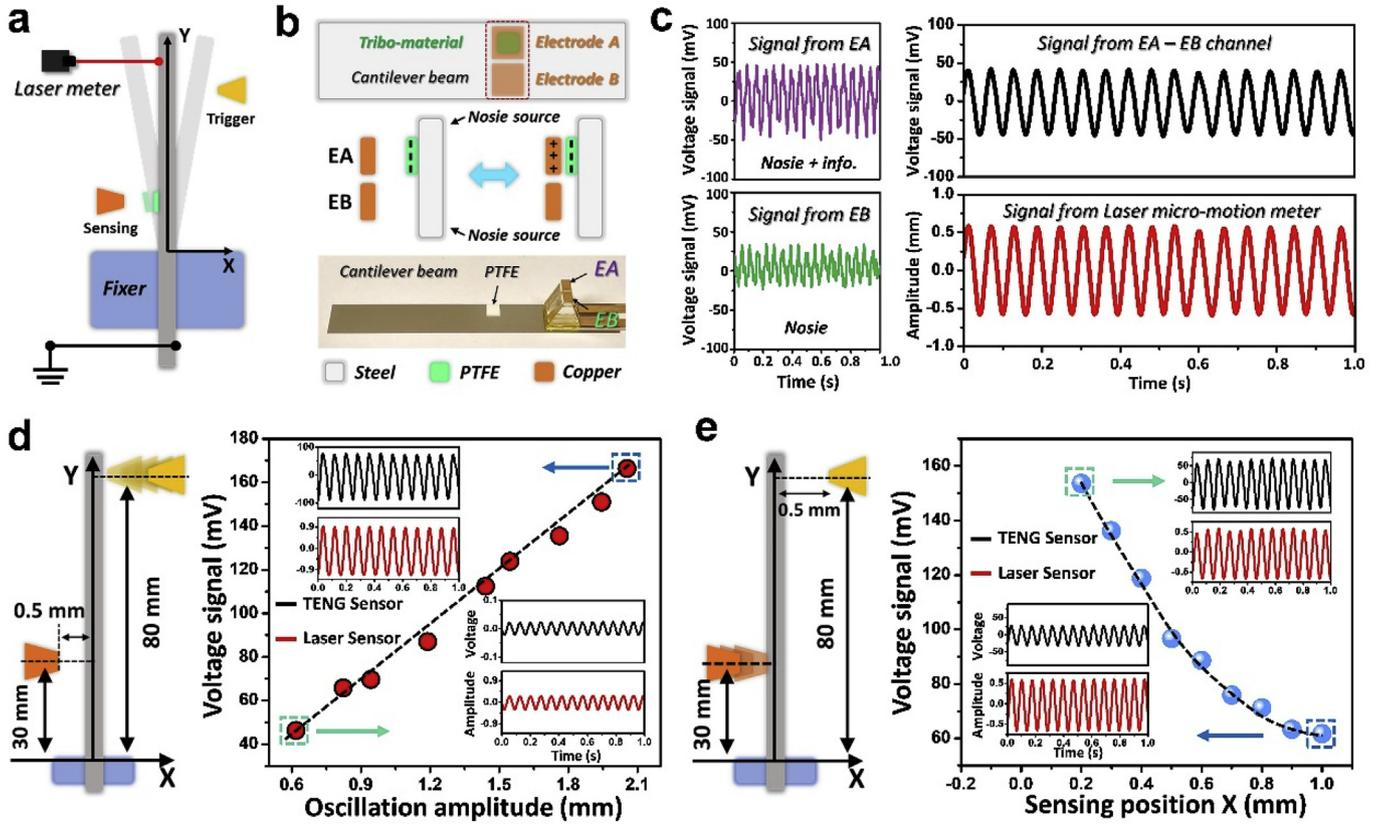
**Fig. 4.** Performance of the real-time oscillation-monitoring sensor (ROS). a) Scheme of the experimental configuration. b) Structure of the single electrode mode triboelectric nanogenerator based micro-motion sensing component. c) Electric signals from EA, EB and EA-EB, and the oscillation amplitude captured by the laser micro-motion meter. d) Electric signal of the ROS under various oscillation amplitudes. e) Electric signal of the ROS under various sensing position X.
