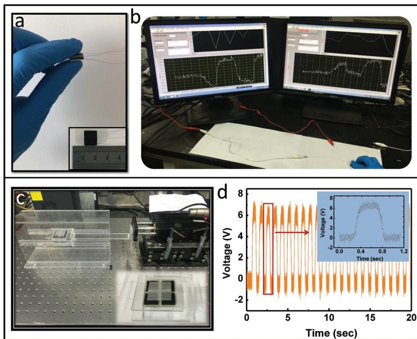
**Figure 6.** Applicability of three-axial force sensor for tactile sensing and mechanical vibration detection. a) Photograph of the mini two-electrode tangential force sensor. b) Screenshot of the real-time output signals of the mini sensor for finger touch detection. c) Platform and system for mechanical vibration detection. d) Output signals of the modified three-axial force sensor for vibration detection.
