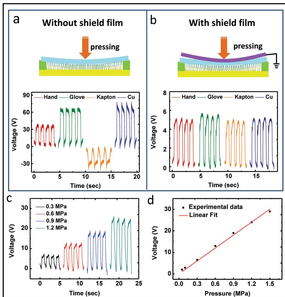
**Figure 2.** Touch detection of the normal force sensor. a,b) Open-circuit voltage when touched by hand, glove, Kapton, and Cu tape of the sensor (a) without shield film (b) with shield film. c) Output performance of the sensor under different pressures. d) The relationship between the output voltages and the applied pressures.
