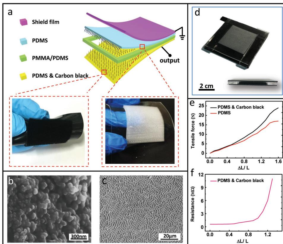
**Figure 1.** Structural illustration of the normal force sensor. a) Schematic diagram of the normal force sensor. b) Micromorphology of carbon black doped in PDMS. c) The surface morphology of the PDMS film. d) Photograph of the sensor. e) Elastic properties of PDMS–CB and original PDMS materials. f) Electrical conductivity of the PDMS–CB material.
