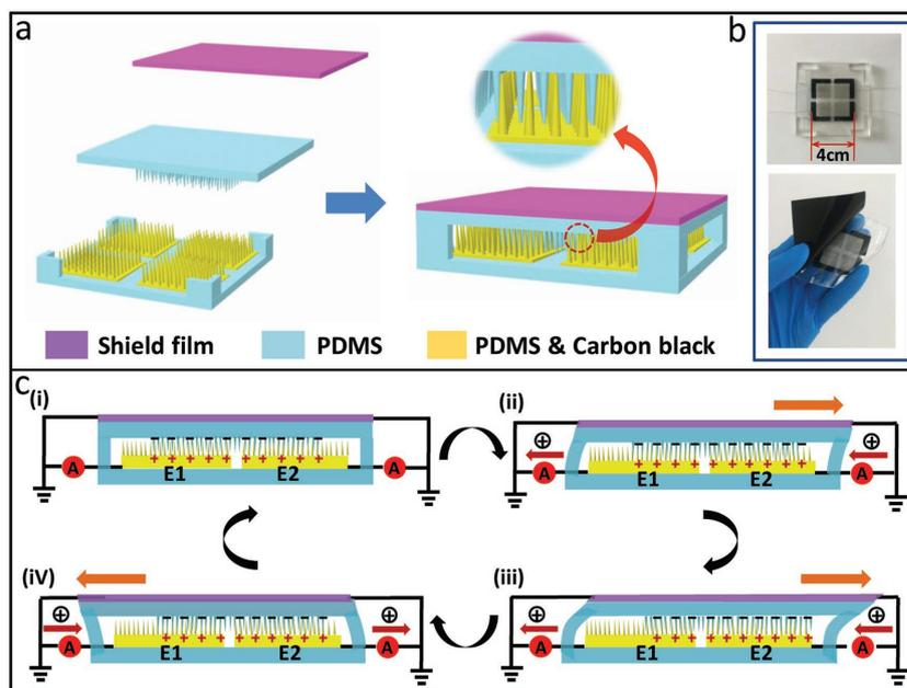
**Figure 3.** Structural illustration of the three-axial force sensor. a) Structure design of the three-axial force sensor. b) Photographs of the three-axial force sensor. c) Detailed mechanism of the voltage generated from the elastic deformation of the dielectric film.
