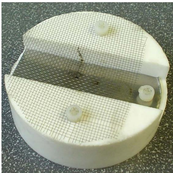
Fig. 2. The electric field generator used in experimentation.
