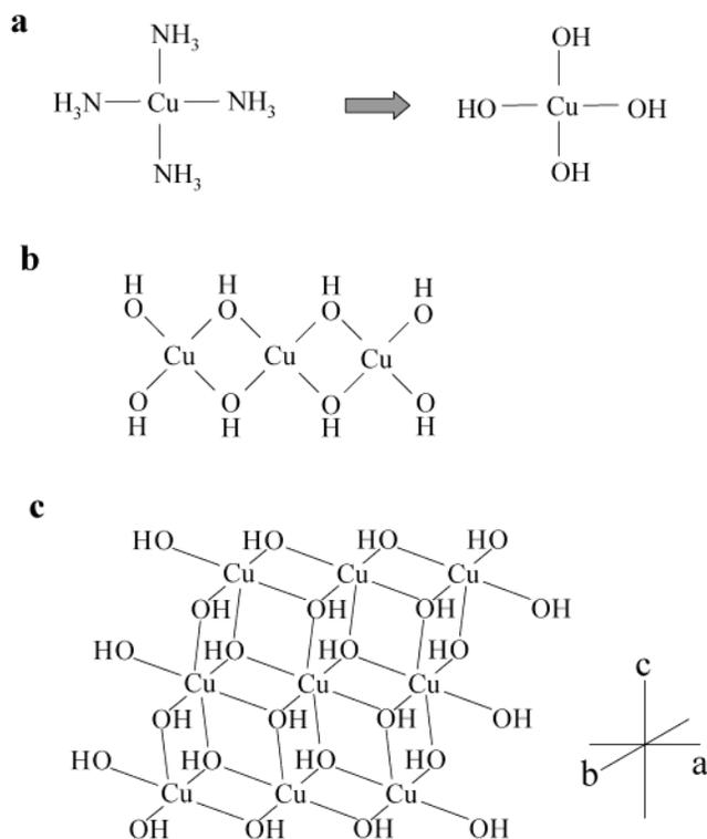
a large surface area and open structure were used as a controlled delivery source of  $\text{Cu}^{2+}$  for the nanoribbon assembly in an aqueous solution under oxidative and alkaline conditions.  $\text{Cu}^{2+}$  was then transported to the assembly sites by  $\text{NH}_3$  in the form of coordination complexes.
