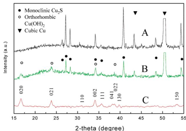
**Figure 1.** XRD patterns of (A) pure  $\text{Cu}_2\text{S}$  nanowires on Cu foil before the growth of  $\text{Cu}(\text{OH})_2$  nanoribbons; (B)  $\text{Cu}(\text{OH})_2$  nanoribbons and the remaining  $\text{Cu}_2\text{S}$  nanowires on Cu foil; and (C) pure  $\text{Cu}(\text{OH})_2$  nanoribbons after separation.
