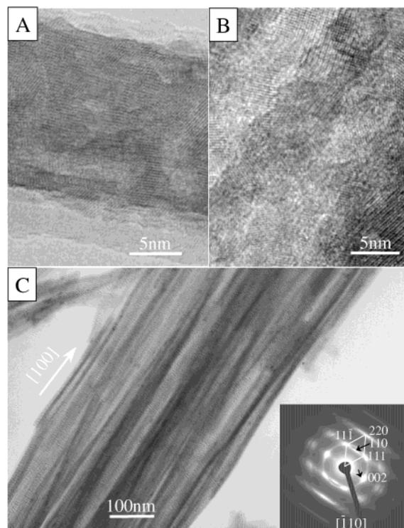
**Figure 3.** HRTEM images of a single nanoribbon of  $\text{Cu}(\text{OH})_2$  (A) and a bundle of nanoribbons (B). (C) A TEM image of bundled  $\text{Cu}(\text{OH})_2$  nanoribbons. Inset of (C): ED pattern of the bundled  $\text{Cu}(\text{OH})_2$  nanoribbons.
