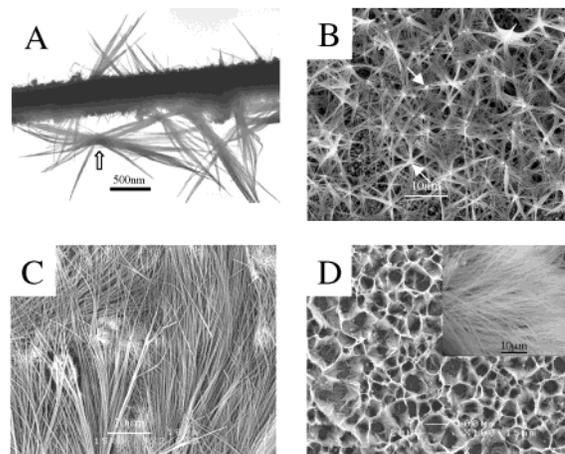
**Figure 4.** TEM and SEM images of  $\text{Cu}(\text{OH})_2$  nanoribbons after different growth times. (A) TEM image after 0.5 h; (B) SEM image after 4 h; (C) SEM image after 3 days; (D) SEM image after 7 days. Inset of (D): higher magnification.
