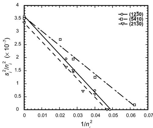
Fig. 5.  $s_i^2/n_i^2$  vs.  $1/n_i^2$  plot for three reflections acquired from the same nanobelt and their linear fits.
