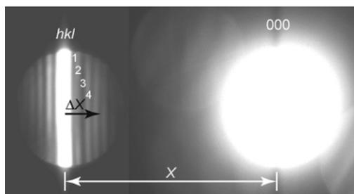
Fig. 2. Illustration of the measurements of  $X$  and  $\Delta X$  in CBED.
