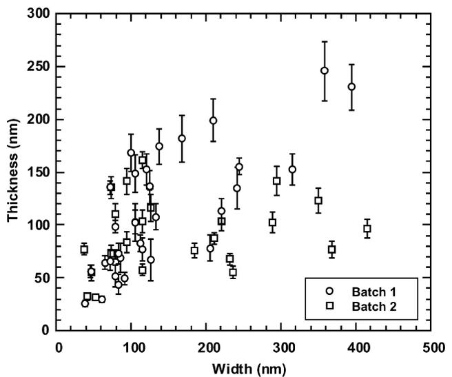
Fig. 7. Measured aspect ratios of nanobelts for two samples as a function of nanobelt widths.
