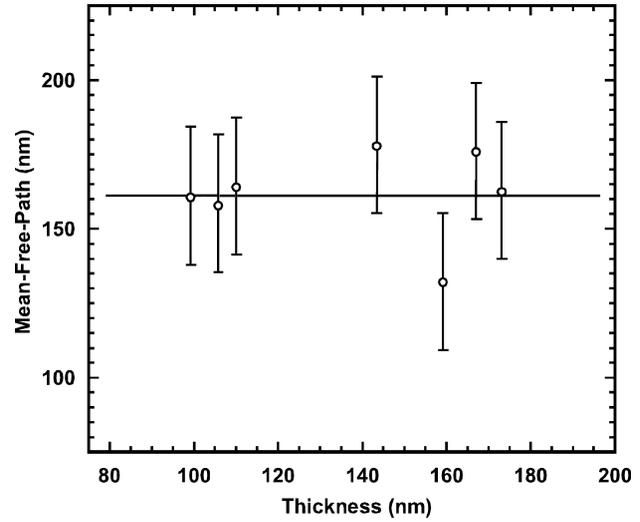
Fig. 6. Plot of experimentally determined mean free path ( $\lambda$ ) values for individual nanobelts versus thickness, showing the data consistency and the independency of  $\lambda$  of the thickness of the nanobelts.
