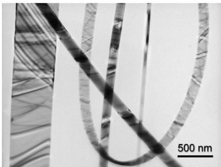
Fig. 1. Typical TEM image of ZnO nanobelts that exhibit a 'ribbon' geometry.
