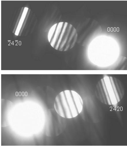
Fig. 4. Two CBED patterns taken from the same nanobelt under two-beam diffracting conditions, which will be used independently for thickness measurements.
