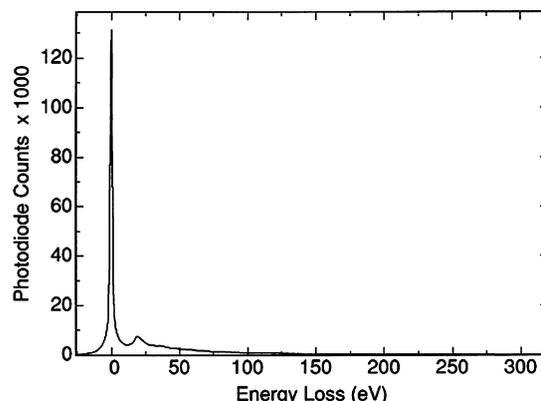
Fig. 3. A typical low-loss EELS spectrum acquired from a ZnO nanobelt at 200 kV.
