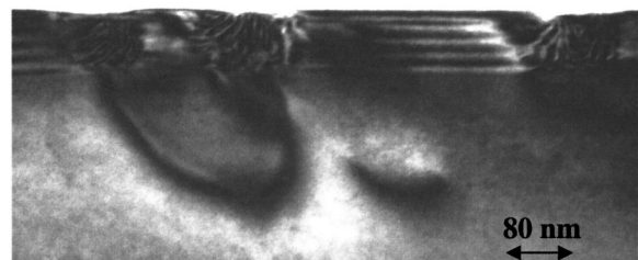
FIG. 2. 3 ML multilayer structure with P 2 anneal at 350 °C.
