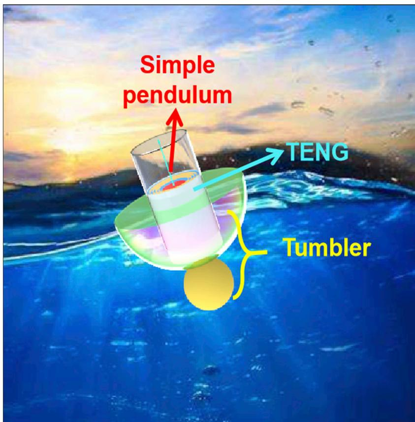
By integrating the tumbler, simple pendulum, and flexible ring triboelectric nanogenerator, the designed active resonance triboelectric nanogenerator can effectively harvest omnidirectional and frequency varying water-wave energy. Thanks to the damped motion of simple pendulum and tumbler, the output performance of AR-TENG system can be greatly improved.
