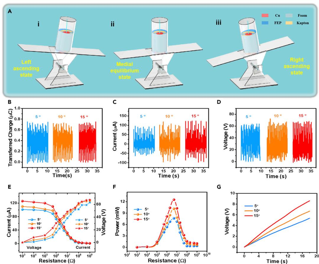
**Figure 3. Output performance of AR-TENG system by driven seesaw**
