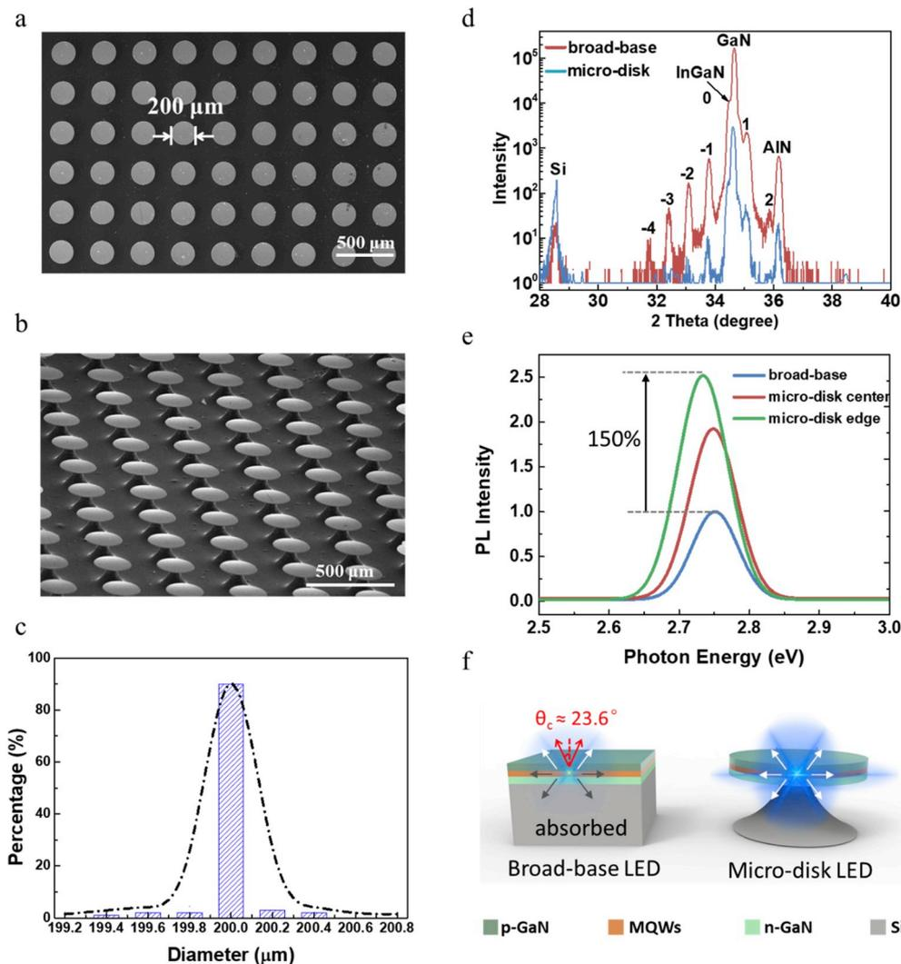
**Fig. 1.** (a), (b) Planar and tilted SEM photographs of InGaN/GaN micro-disk LED array. (c) Statistical distribution of diameters of the micro-disk LEDs. (d) XRD  $\omega$ -2 $\theta$  curve for InGaN/GaN micro-disk LED array. (e) PL spectra for micro-disk LED and broad-base LED. (f) Schematic diagram of the effective light emission region for broad-base LED and micro-disk LED.
