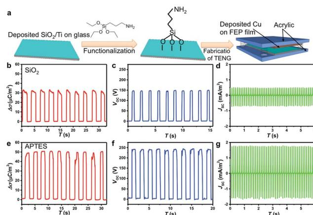
Fig. 6 SAM surface functionalization of  $\text{SiO}_2$  as the triboelectric layer in TENGs to enhance the output performance. (a) Fabrication process and (b–g) output performances of the TENGs with pristine and functionalized silica (10% APTES in volume ratio). (b–d) and (e–g) show the measured charge density, the open-circuit voltage and the short-circuit current density of TENGs with the pristine and functionalized silica, respectively.
