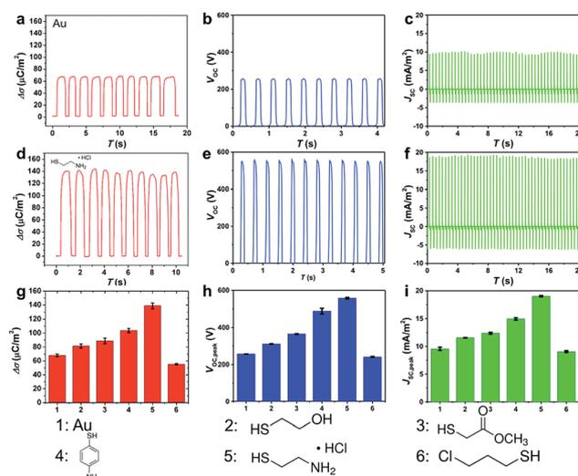
Fig. 4 Output performance of the TENGs with pristine (#1) and functionalized Au (#2–6) surfaces. (a–c) and (d–f) show the measured transferred charge density ( $\Delta\sigma$ ), the open-circuit voltage ( $V_{OC}$ ) and short-circuit current density ( $J_{SC}$ ) of the #1 and #5 TENGs, respectively. (g–i) show the comparisons of the transferred charge density, open-circuit voltage and short-circuit current density of all the 6 TENGs.
