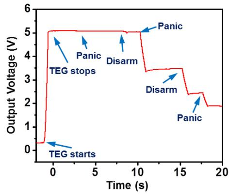
**Supplementary Figure 5 | Output voltage of the power-supplying system when powering a wireless emitter.** For the triboelectric generator rotating for less than 1 sec at  $3000 \text{ rmin}^{-1}$ , the system can sustain 5 times of wireless transmission, which enables the alarm to switch between “panic” state and “disarm” state.
