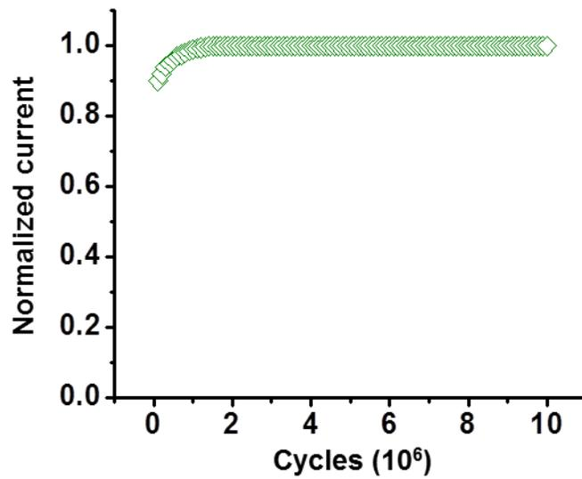
**Supplementary Figure 3 | Normalized current as a function of operation cycles.** At the beginning, the increasing current is due to the accumulation of triboelectric charges. After the triboelectric charging saturate, the current output becomes stable.
