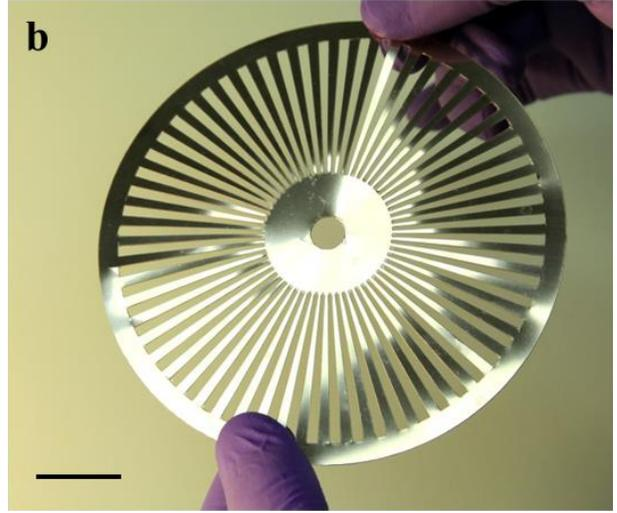
**Supplementary Figure 8 | A thin-film based triboelectric generator fabricated on flexible polyamide substrate. a and b are stator (scale bar: 2cm) and rotator (scale bar: 2cm), respectively.**
