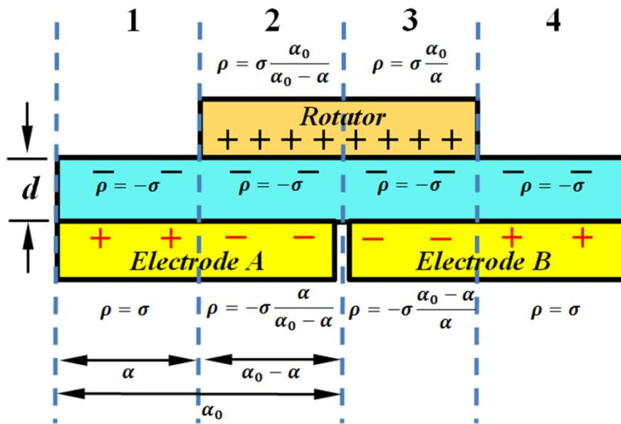
Supplementary Figure 1 | Schematic illustration of a cross-sectional view of charge distribution in open-circuit condition at the intermediate state.
