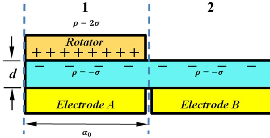
Supplementary Figure 2 | Schematic illustration of a cross-sectional view of charge distribution in open-circuit condition at the initial state.
