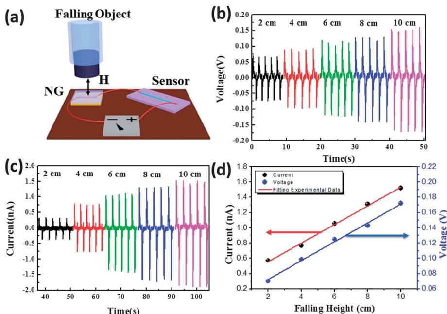
**Fig. 4** (a) Schematic diagram of the nanogenerator testing method. (b and c) The output voltage and current of the nanogenerator under impact (0.33 Hz) exerted by a free-falling object with different heights of 2, 4, 6, 8, and 10 cm; the object weighed 300 g. (d) The output voltage and current as function of varied height; experimental and fitting curves.
