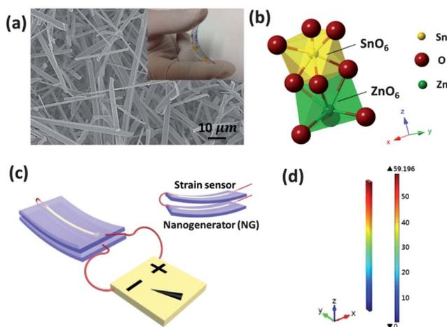
**Fig. 1** (a) FESEM image of ZnSnO<sub>3</sub> microbelts. Inset image is a digital micrograph of the nanogenerator/strain sensor. (b) Atomic model of the rhombohedral structure ZnSnO<sub>3</sub>. (c) The schematic diagram of the self-powered strain-sensing system made from a nanogenerator and strain sensor. (d) Theoretical calculation of the piezoelectric potential distribution in a ZnSnO<sub>3</sub> microbelt under an axial compressive stress.
