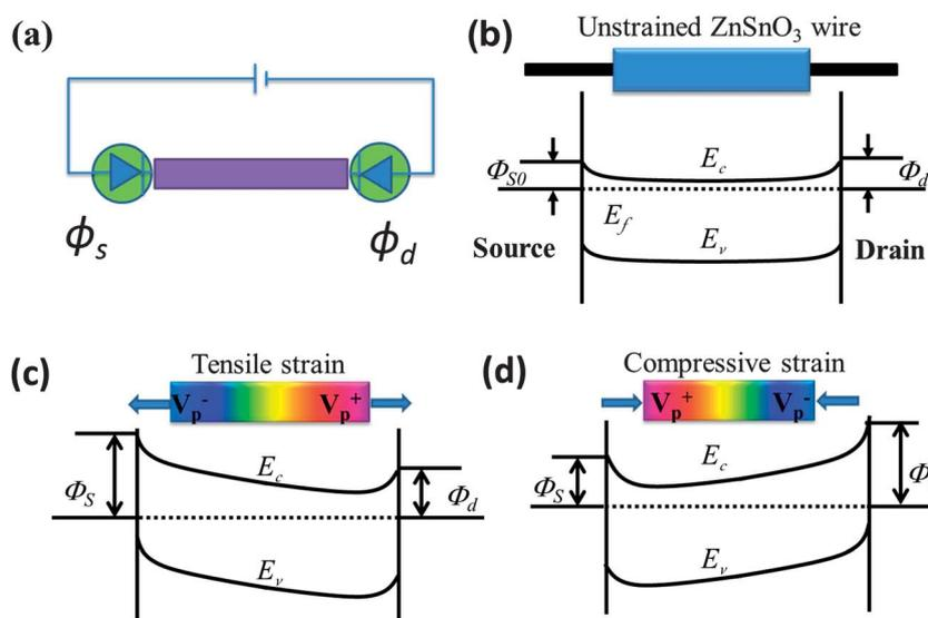
**Fig. 3** Energy band diagram presents the asymmetric SBH at the source and drain contacts of a single-belt  $\text{ZnSnO}_3$  (a) A back-to-back with SBH of a sensor made from  $\text{ZnSnO}_3$ , which is subjected to (b) no strain, (c) tensile strain, and (d) compressive strain. These illustrate the piezopotential of the microbelt can be finely tuned by varied strains.
