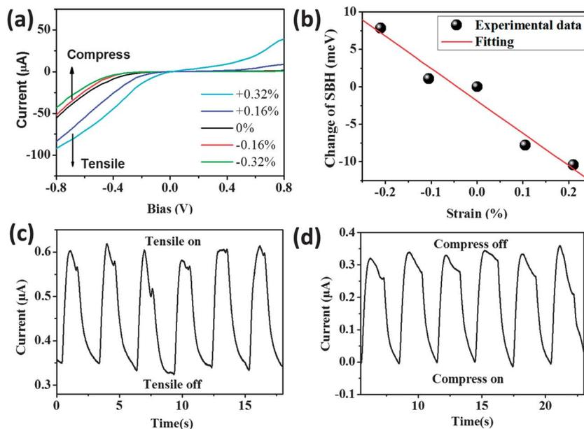
**Fig. 2** (a)  $I$ - $V$  characteristic of a strain sensor under varied compressive and tensile strains. (b) By utilizing the thermionic emission-diffusion model to estimate the change in SBH as a function of varied strain. (c) Current response of a strain sensor that was repeatedly by a tensile and (d) compressed stress.
