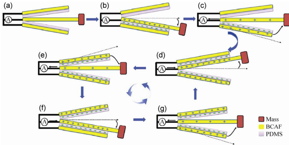
**Figure 2** A cycle of electricity generation process for illustrating the mechanism of the triple-cantilever based TENG (see text). (a) Original position without vibration; (b) and (c) initial steps for generating the triboelectric charges via contact induced electrification. (d)–(g) Repeated processes for power generation during a cycled vibration of the cantilever.
