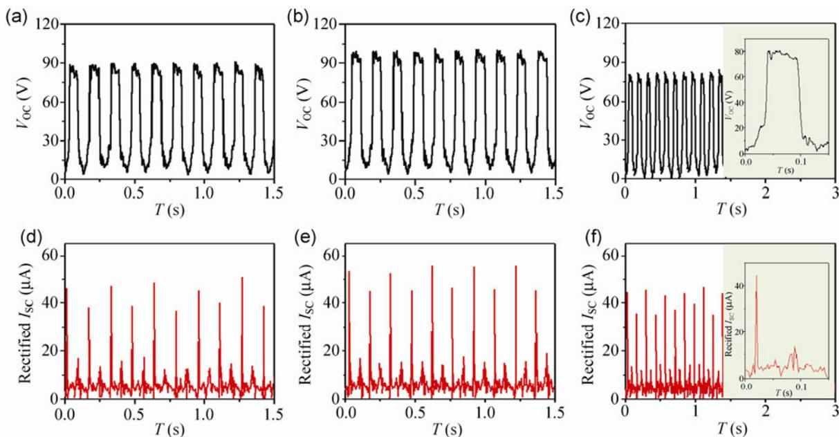
**Figure 3** Open-circuit voltage ( $V_{OC}$ ) at vibration frequencies of 3.5 Hz (a), 3.7 Hz (b), and 4.0 Hz (c) and rectified short-circuit current ( $I_{SC}$ ) at vibration frequencies of 3.5 Hz (d), 3.7 Hz (e), and 4.0 Hz (f). The insets of (c) and (f) are enlarged views of half cycles of the  $V_{OC}$  and  $I_{SC}$  at 4.0 Hz, respectively.
