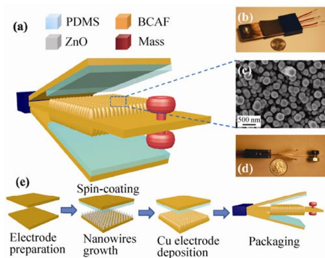
**Figure 1** (a) Sketch and (b), (d) photographs of a typical triple-cantilever based TENG, with a size equivalent to a quarter dollar coin. (c) Scanning electron microscopy (SEM) image of Cu film coated ZnO nanowire arrays. (e) Fabrication process of the TENG.
