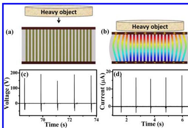
**Figure 2.** Working principle and performance of the NG. (a) Schematic diagram of NG's structure without deformation. (b) A schematic picture of the piezoelectric potential distribution in a deformed NG when suffer an impact force. The red and blue color regions indicate a positive and negative piezoelectric potential, respectively. (c) Output voltage and (d) output current of the NG under a periodic pressure of 0.53 MPa.
