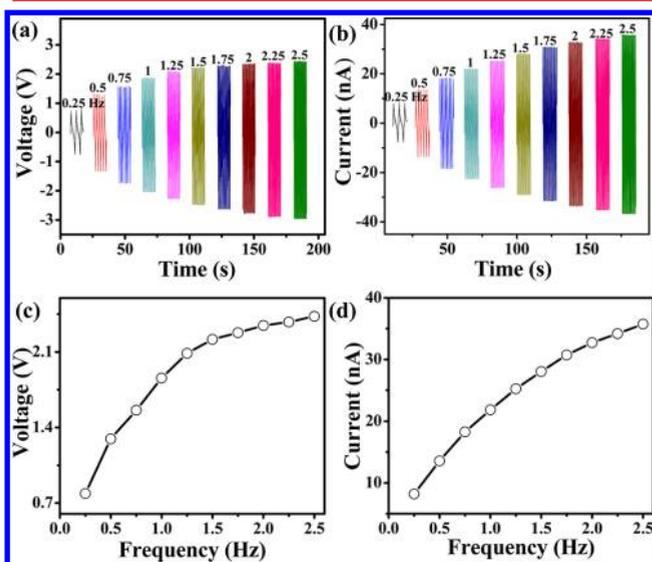
**Figure 5.** Performance of the NG under different impact frequencies. (a,b) The output voltage and output current of the NG under different frequencies ranging from 0.25 to 2.5 Hz. (c,d) Relationship between the peaks of the output voltage (output current) and the impact frequencies.
