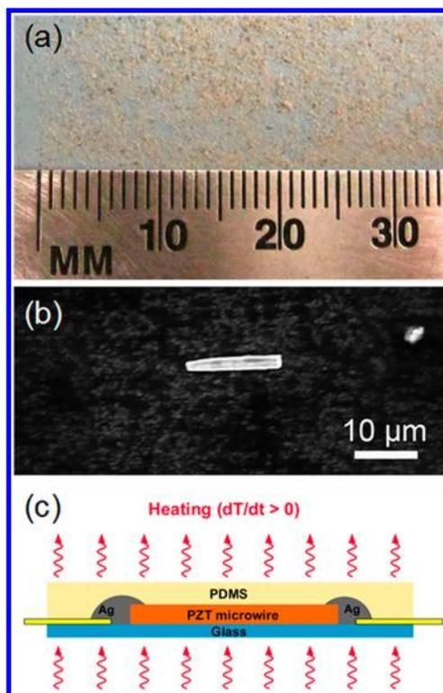
**Figure 1.** (a) Photograph of the obtained PZT micro/nanowires. (b) SEM image of a single PZT microwire. (c) Schematic diagram showing the structure of a single PZT microwire pyroelectric nanogenerator.
