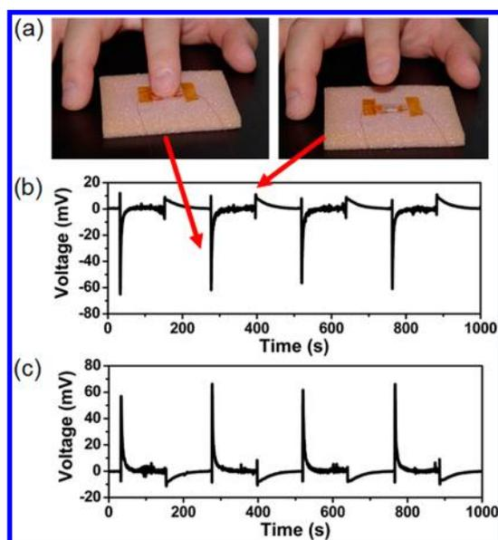
Figure 5. (a) The optical images when a finger touched the fabricated sensor and was then moved out. (b) The  $V-T$  curve when the finger touched the sensor in four times under the forward connection condition. (c) The corresponding  $V-T$  curve under the reversed connection condition.
