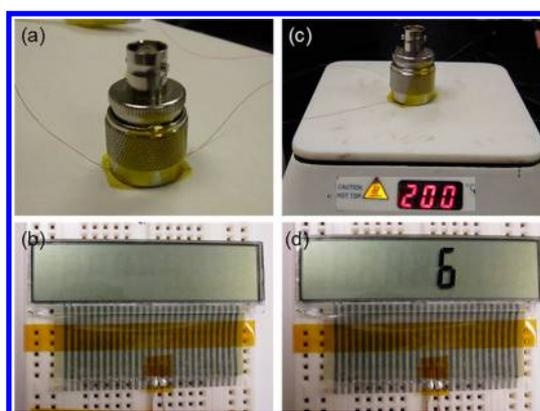
Figure 6. (a) The optical image when a self-powered sensor was attached on a metallic body. (b) The optical image of a LCD screen, which is connected to the sensor in panel a. (c) The optical image when the sensor is in contact with a hot-plate with the temperature of 473 K. (d) The optical image of the lighted LCD screen, which is connected to the pyroelectric generator in panel c.
