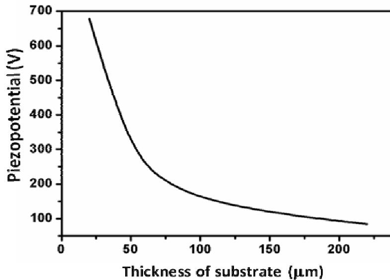
**Fig. S2.** Calculated piezopotential between the top and bottom electrodes as a function of the thickness of the substrate while the applied stress is fixed. When the length of the nanowire is kept at 2 mm, if we fix the applied stress at 8 MPa, the calculated piezopotential difference between the top and bottom electrode increases as the thickness of substrate is reduced.
