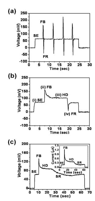
**Fig. 3** Hybrid operation by solar energy (SE) and mechanical energy with controlled mechanical straining processes. Under the 'solar' energy given by indoor light, the overall output voltage by controlled mechanical straining processes of (a) fast bending (*FB*) and fast releasing (*FR*), (b) *FB*, holding (*HD*), and *FR*, and (c) *FB*, *HD*, and slow releasing (*SR*).
