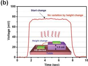
**Fig. 6** Verification of solar power variation according to the angle and height changes of a device (a) output voltage by solar energy according to the angle change of a hybrid device and (b) output voltage by solar energy according to the height change of a hybrid device. We can clearly confirm that the sharp output responses (see Fig. 3) by bending together with solar energy originated from the piezoelectric field in ZnO.
