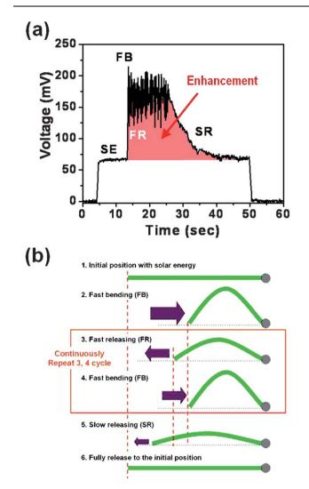
Fig. 5 Synergetic enhancement by the contribution of the piezoelectric element during solar power generation. (a) Output voltage measured by controlling straining processes under solar energy (SE) with fast bending (FB), fast release (FR), but not fully release, and slow releasing (SR). (b) The detailed straining process. The green part is our hybrid device.
