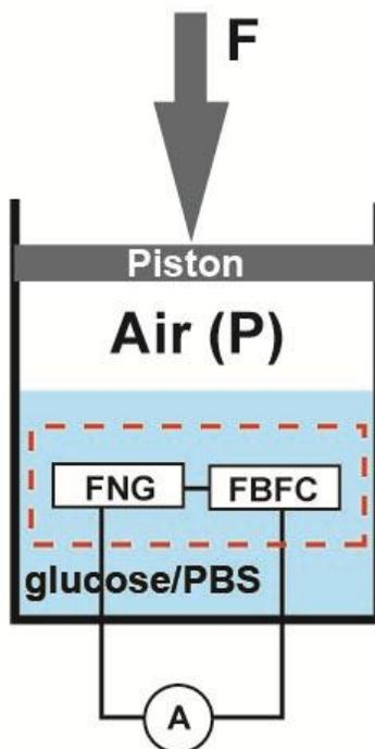
**Fig. S5.** In the experiment, the hybrid nanogenerator is immersed in glucose/PBS solution inside a closed container, as shown in the figure. When a periodic force is applied onto the piston, the air in the closed container is compressed; as a result, the pressure applied on the solution (also on the devices) increases, the current in the circuit increases. When the pressure is released, a rapid and obvious decrease in current is detected, as shown in Fig. 3 and Fig. 4.
