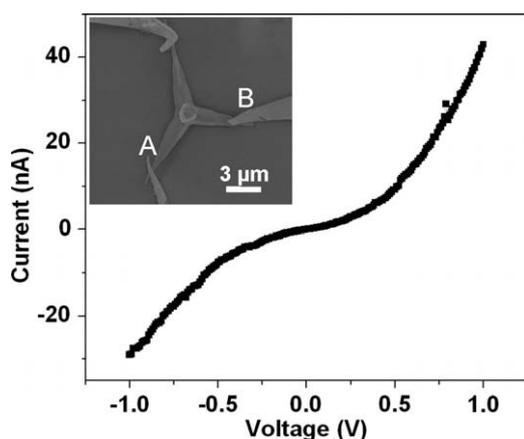
**Fig. 1.** Typical  $I$ - $V$  characteristic of ZnO tetrapod measured by using tungsten (W) tips directly in contacting with the branches. Inset is an SEM image of the measured ZnO tetrapod.
