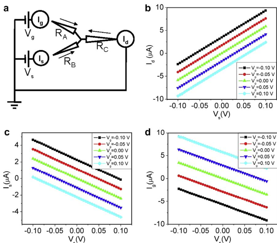
**Fig. 4.** (a) Schematic circuit for the measurement of “gating” effect of a ZnO tetrapod. The current flowing through (b) drain, (c) source and (d) gate electrode at different gating voltages.
