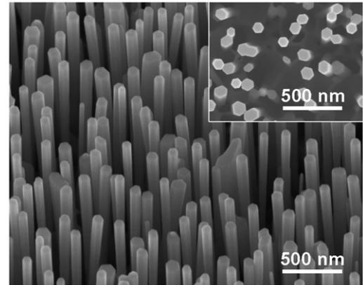
Fig. 2. A 30° tilted view SEM image of the zinc oxide nanowire arrays. Inset: top-view SEM image of the zinc oxide nanowire arrays.
