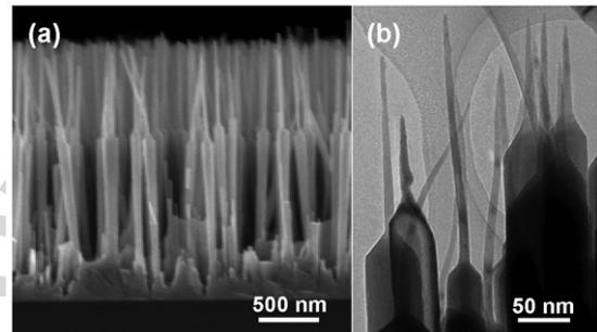
Fig. 3. (a) Cross-section view SEM image of the vertical aligned ZnO nanotip arrays. (b) Low magnification TEM image of the ZnO nanotips.
