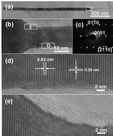
Fig. 4. (a) Low magnification TEM image of an individual ZnO nanotip. (b) Enlarged TEM image from the rectangle-enclosed area of (a). (c) Corresponding SAED pattern of the ZnO nanotip indicates the ZnO nanotip is single crystalline with [0001] growth direction. (d) High resolution TEM image of the tip region of the zinc oxide nanotip corresponding to the rectangle region *D* in (b). (e) High resolution TEM image of the shoulder region that was taken from the rectangle region *E* in (b).
