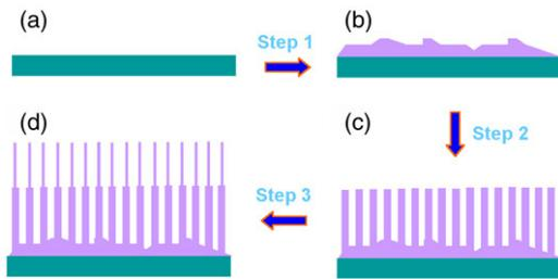
Fig. 1. Schematic diagram of the growth process for the aligned ZnO nanotip arrays.
