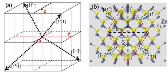
FIG. 3. (Color online) (a) Sketch of the four equivalent directions  $[111]$ ,  $[\bar{1}\bar{1}\bar{1}]$ ,  $[1\bar{1}\bar{1}]$ , and  $[\bar{1}\bar{1}1]$  for the cubic ZB structures. (b) The atomic model of ZB structure projected along the  $[011]$  direction.
