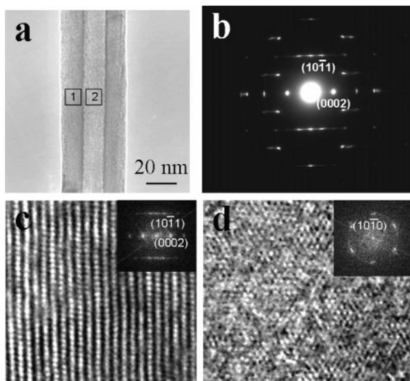
**Figure 2.** Structural analysis of the monochiral MWCNTs. (a) TEM image. (b) Electron diffraction pattern. (c) and (d) High-resolution TEM images corresponding to the areas marked by B and C in (a), respectively. FFT images (inset in (c) and (d)) reveal the consistent pattern with the experimental.
