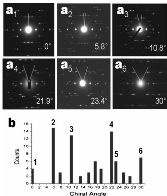
**Figure 3.** (a) Series of typical electron diffraction patterns of MWCNTs with chiral angles of 0°, 5.8°, 10.8°, 21.9°, 23.4°, and 30°, respectively. (b) Statistical histogram showing the distribution of the chirality for the 82 as-prepared MWCNTs; the columns marked by 1–6 correspond to  $a_1$ – $a_6$  in (a), respectively.
