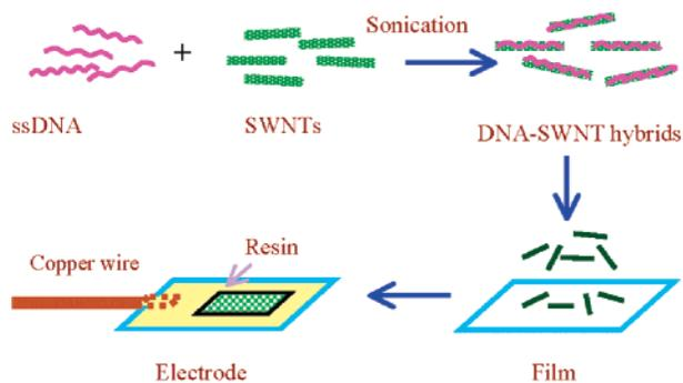
**Figure 1.** The fabrication process of DNA–SWNT electrode. First, ssDNA was mixed with SWNT to form DNA–SWNT hybrid, and then, the DNA–SWNT hybrids were deposited onto a glass substrate to form a uniform film, and finally, the film was welded with copper wire and mounted with resin, leaving a small nanotube area for sensing.
