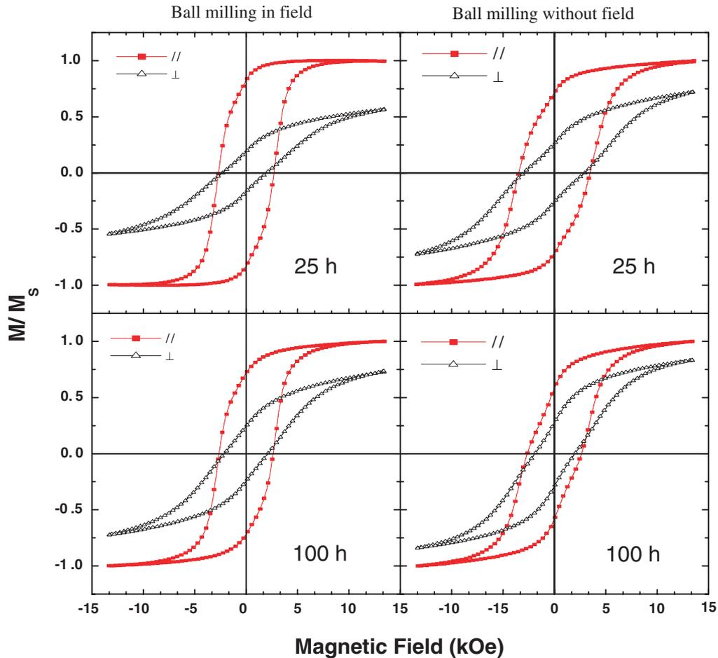
**Figure 1.** Magnetic hysteresis loops measured in both the alignment direction (easy magnetization direction) and the direction perpendicular to the easy direction of  $\text{Nd}_2\text{Fe}_{14}\text{B}$  powder samples aligned in solidified epoxy. The left column has loops of the powders milled in a magnetic field and the right column has loops of the powders milled without a magnetic field.
