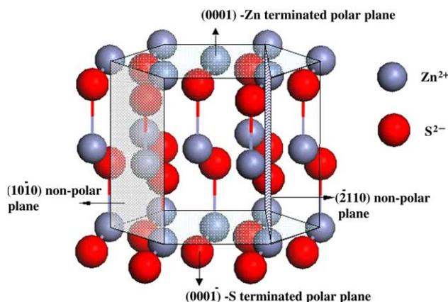
Fig. 3. Structure model of wurtzite ZnS.
