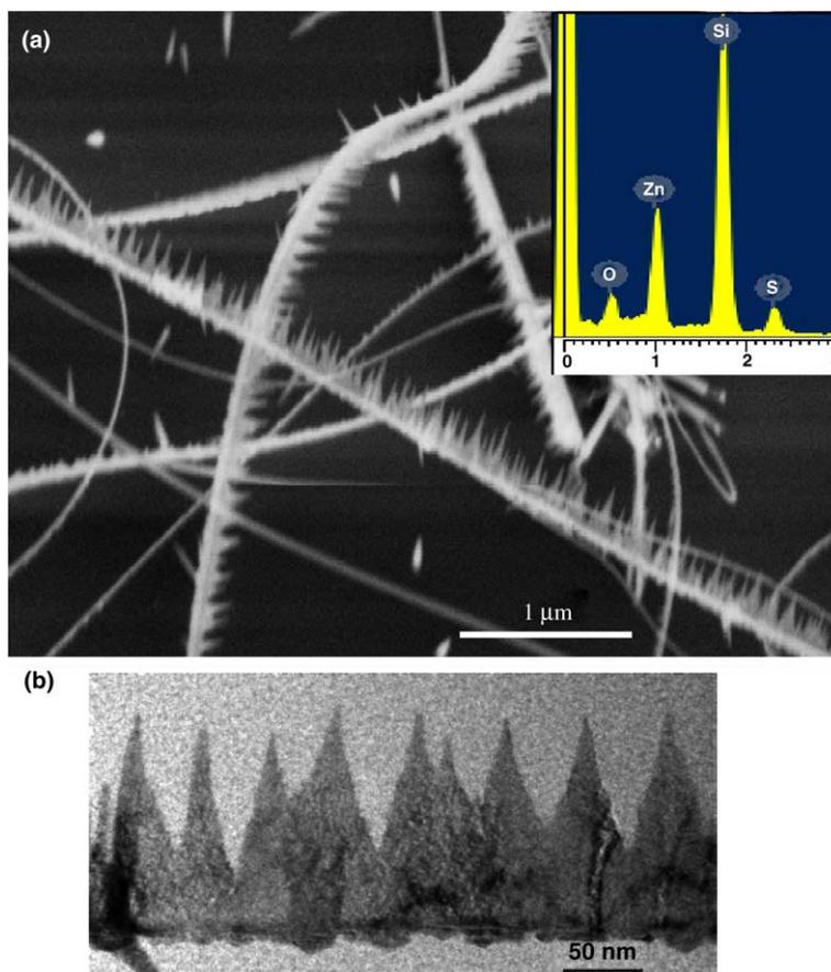
Fig. 1. (a) SEM image of the as-synthesized ZnS nanostructures. The inset is an energy dispersive X-ray spectrum recorded from the sample. (a) The Zn and S peaks are due to the nanostructures, while the silicon and oxygen peaks are due to the silicon substrate.
