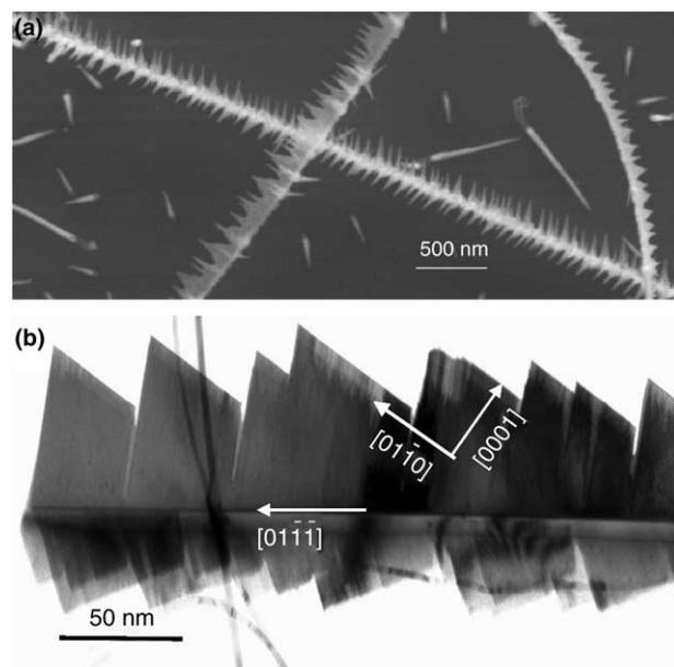
Fig. 4. (a) 'Feather' structure of ZnS. (b) A TEM image of the feather structure and the corresponding growth directions.
