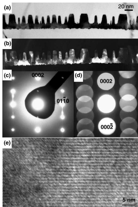
Fig. 2. (a) Bright field TEM image of a ZnS nanosaws. The polar growth occurs mainly on one side of the belt. (b) Dark field TEM image of the saw structure. (c) Diffraction pattern shows the saw ribbon is along  $[0\bar{1}\bar{1}0]$  and the saw-teeth are along  $[0001]$ . (d) CBED pattern recorded from the sample. (e) High-resolution TEM image recorded from the ZnS nanosaw.
