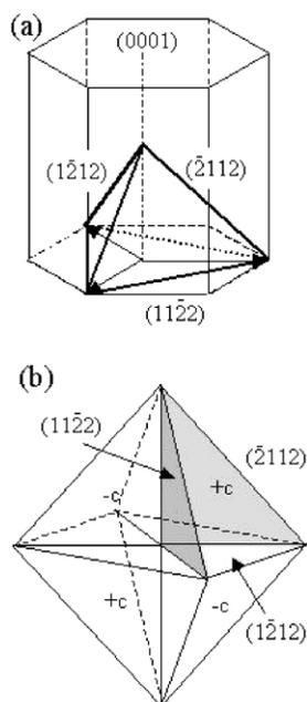
Fig. 4. (a) A pyramid formed by three  $\{11\bar{2}\}$  and one (0001) facets. (b) The octa-twin model composed of eight pyramidal inversion-twin crystals [27].
