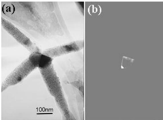
Fig. 2. (a) Bright-field electron micrograph of a tetraleg ZnO nanostructure. (b) A dark-field electron micrograph from the same region, showing a distinct grain at the center, which will be explained by the model presented in Fig. 4(b).
