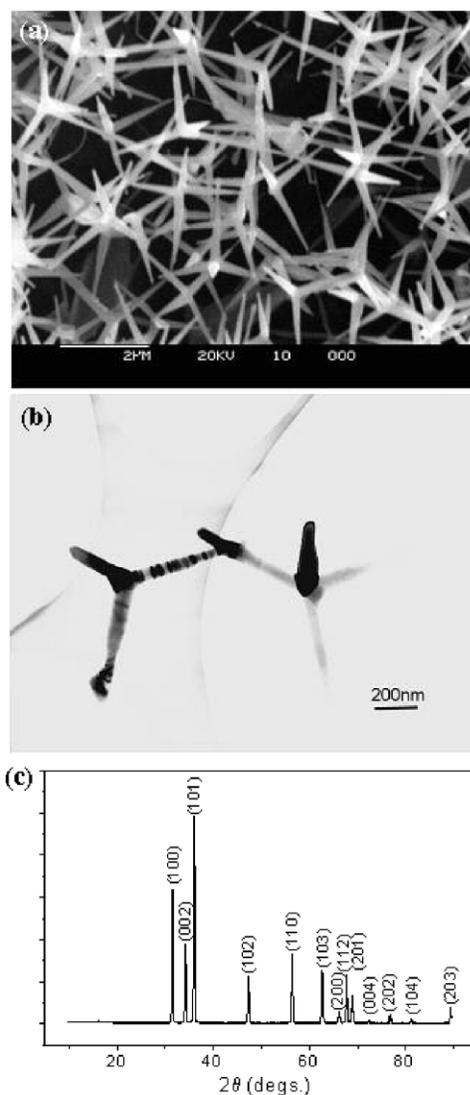
Fig. 1. (a) A typical SEM image showing the general morphology of the tetraleg ZnO nanostructure. (b) An TEM image of the tetraleg structure. (c) XRD pattern from the tetraleg ZnO nanostructure, showing the Wurtzite structure.
