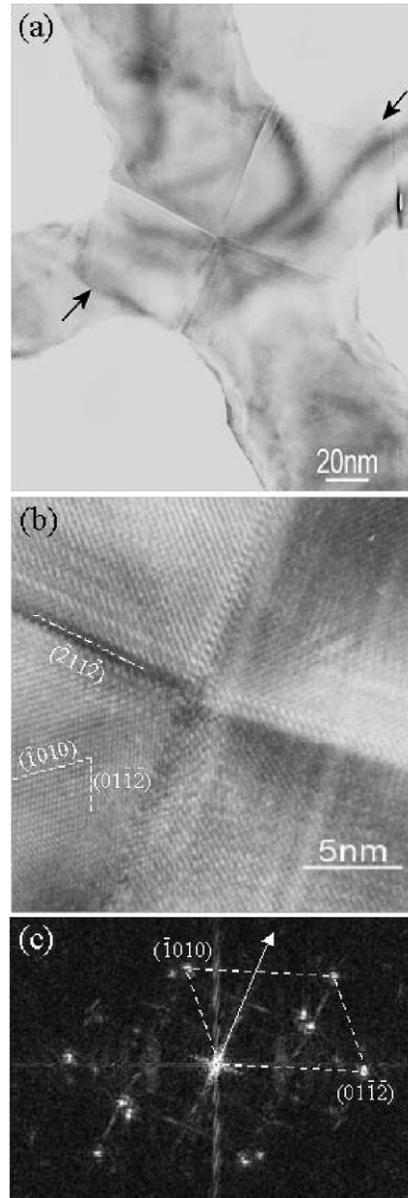
Fig. 3. (a) Low magnification TEM image of a tetraleg ZnO nanostructure. (b) A high-resolution TEM image recorded from the center of the tetraleg structure. (c) A Fourier transform of the image given in (b) and the indexes corresponding to one of the bottom-left grain in (b). The incident beam direction is  $[24\bar{2}3]$ .
