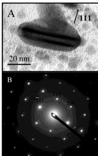
**Figure 4.** (A) TEM image of the silver nanodisk taken in side view, showing the contrast from (111) stacking faults and a preferential growth along the stacking faults. The orientation relationship of the SAED pattern and the nanodisk is shown in Figure 3, parts A and B. (B) A typical SAED pattern of silver nanodisk at 100 kV in the  $[01\bar{1}]$  orientation (side view).
