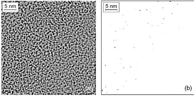
FIG. 3. (a) Same image as Fig. 1(a), Fourier-filtered using a passband of  $0.5\text{--}1.4\text{ nm}^{-1}$ . (b) Same image as (a), with a threshold chosen to reveal features with brightness three standard deviations greater than the mean. The contrast in this image was inverted for improved reproduction, so that bright features from (a) appear dark here.
