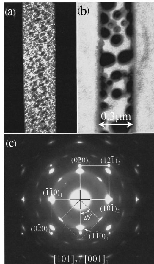
FIG. 3. (a) Dark-field TEM image of a  $\text{PbO}_2$  nanobelt post to electron beam irradiation, where the mottled contrast indicates occurrence of precipitation. (b) Bright-field TEM image of a  $\text{PbO}_2$  nanobelt after undergoing a long time irradiation, in which  $\text{PbO}_2$  has decomposed into metal Pb; (c) electron diffraction pattern of the nanobelt shown in (a), displaying the phase transformation from  $\text{PbO}_2$  to  $\text{PbO}$ .
