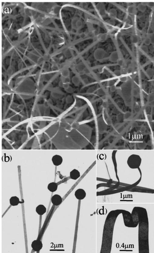
FIG. 1. (a) SEM image of the as-synthesized  $\text{PbO}_2$  nanobelts and Pb particles; (b)–(d) are bright-field TEM images of the  $\text{PbO}_2$  nanobelts, showing that each nanobelt has a Pb tip, and (c)–(d) display the twist feature of the nanobelt.
