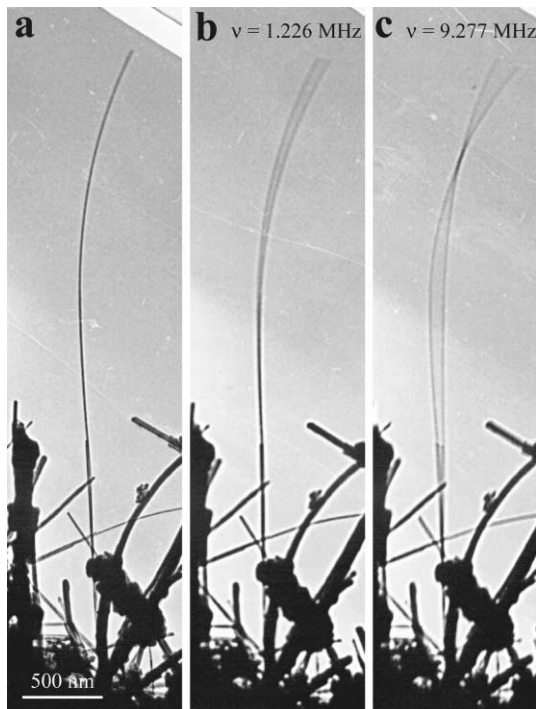
Fig. 3. A bent carbon nanotube at (a) stationary, (b) the first and (c) the second harmonic resonance induced by an externally applied electric field.
