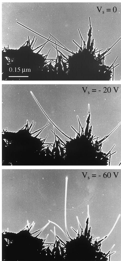
Fig. 5. Electrostatic deflection of a carbon nanotube induced by a constant field across the electrodes. Quantification of the deflection gives the electrical charge on the carbon nanotube and the mechanical strain on the fiber.
