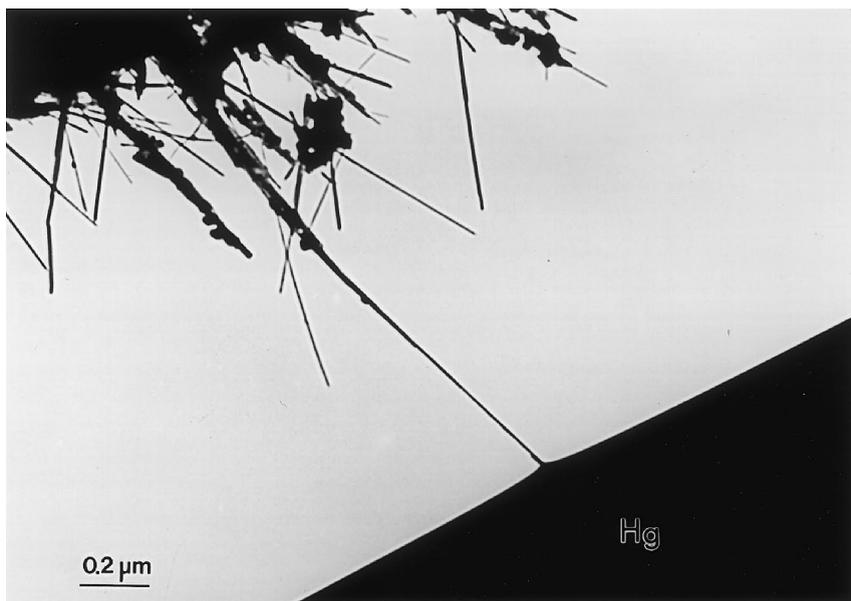
Fig. 3. In situ TEM image showing the contact of a carbon nanotube with a liquid mercury during the electric transport measurement.
