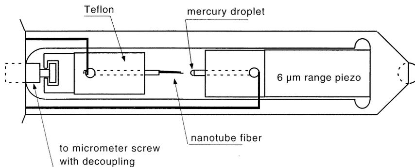
Fig. 1. Schematic diagram of the newly built TEM specimen holder for in situ measurement the mechanical properties of a single nanofiber.
