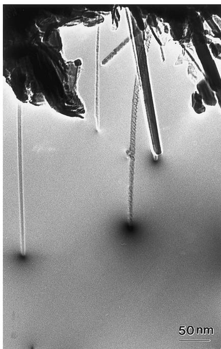
Fig. 8. In situ TEM observation the electric field induced electron emission from carbon nanotubes. The applied voltage is 60 V and the emission current  $\sim 20 \mu\text{A}$ .
