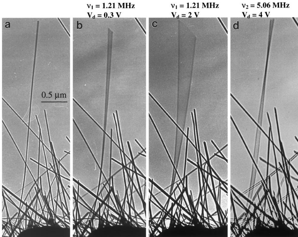
Fig. 6. A selected carbon nanotube at (a) stationary, (b,c) the first harmonic resonance ( $\nu_1 = 1.21$  MHz) and (d) the second harmonic resonance ( $\nu_2 = 5.06$  MHz).  $V_d$  is the magnitude of the applied voltage.
