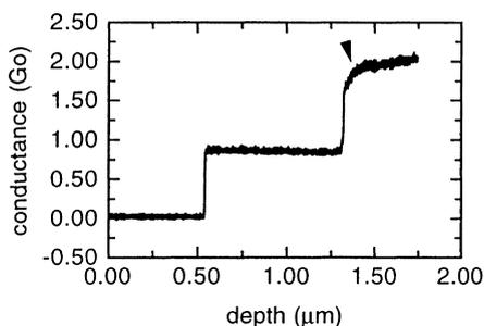
Fig. 4. Conductance of carbon nanotubes observed using the set up in an AFM, showing the independence of the conductance on the depth into the liquid mercury the tip being inserted. The second stair is introduced as another nanotube touches the mercury.
