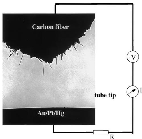
Fig. 2. TEM image showing carbon nanotubes at the end of the electrode and the other count electrode. A constant or alternating voltage can be applied to the two electrodes to induce electrostatic deflection or mechanical resonance.
