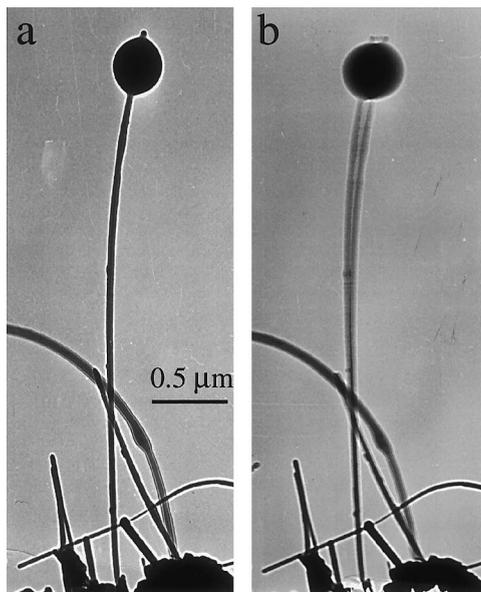
Fig. 7. A small particle attached at the end of a carbon nanotube at (a) stationary and (b) first harmonic resonance ( $\nu = 0.968$  MHz). The effective mass of the particle is measured to be  $\sim 22$  fg ( $1 \text{ f} = 10^{-15}$ ).
