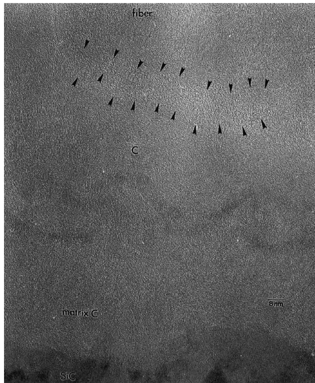
Fig. 4. A high-magnification TEM image of carbon-carbon interfacial zones showing graphitic layers of fiber (F), fiber coating (C), and matrix layers of C and SiC.
