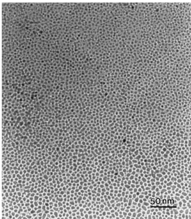
Figure 1. Self-assembly of the size unselected cobalt nanocrystals (4–9 nm), showing size differentiation in the perpendicular drying process.
