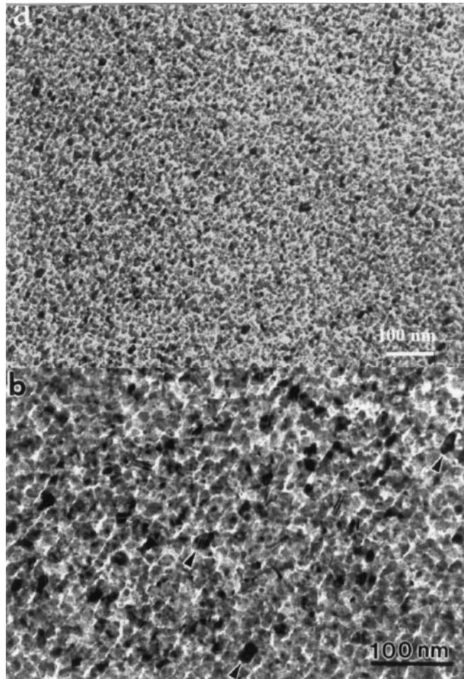
Figure 5. One dimensional self-assembly of cobalt nanocrystal arrays with sizes of 10–20 nm. (a) A low magnification view and (b) a higher magnification view showing the anisotropy shapes of the ferromagnetic nanocrystals. The arrowheads indicate the alignment of the longitudinal directions of the particles with the assembling direction.
