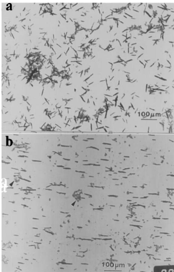
Figure 3. (a) Optical micrograph of the as-prepared cobalt nanoparticle composites, showing the formation of anisotropy whiskers in the solution and the random orientation of the whiskers. (b) Optical micrograph of the whiskers deposited on a glass plate with the presence of a magnetic field during the drying process, showing the alignment of the whiskers along the field direction.
