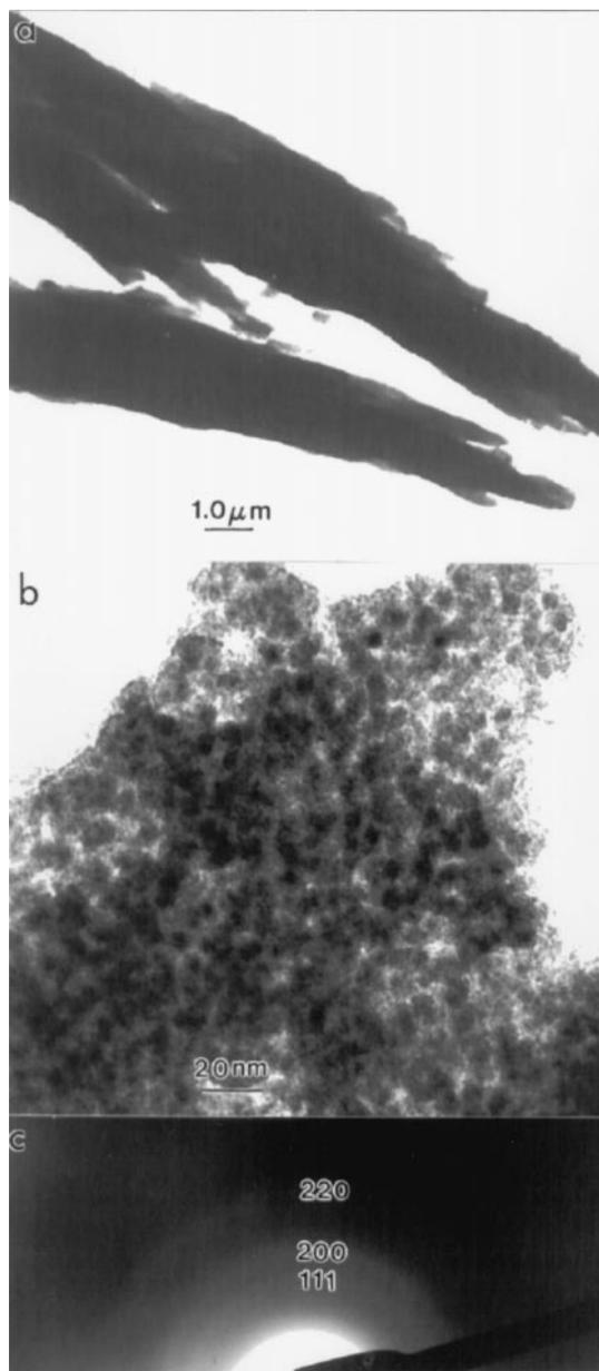
Figure 4. (a) A low magnification TEM image of the whiskers, (b) an enlarged TEM image of a whisker showing the cobalt nanoparticles with sizes of 5–8 nm, and (c) an electron diffraction pattern recorded from cobalt particles illustrating the face-centered cubic structure of the particles. The diffraction pattern is diffuse because of the presence of polymer and the low processing temperature.
