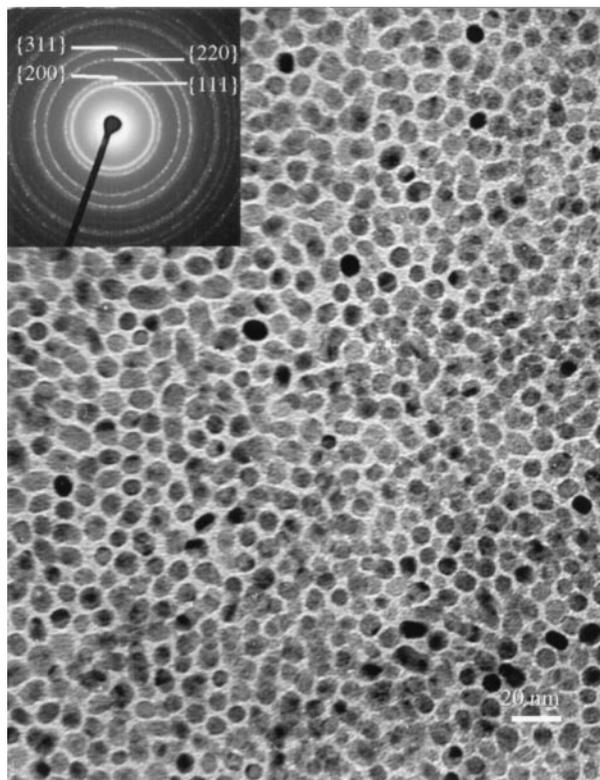
Figure 2. Ordered self-assembly of cobalt nanocrystals. The inset is an electron diffraction pattern (SAD) from the nanocrystals showing the face-centered cubic structure.
