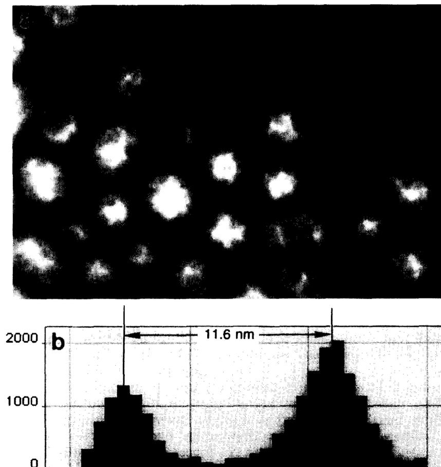
Fig. 6. (a) A background subtracted 15 eV plasmon-loss energy-filtered TEM image showing only the contribution of the metallic Al (b) A line scan across particle A (indicated in (a)) for the estimation of the thickness of the Al wall.
