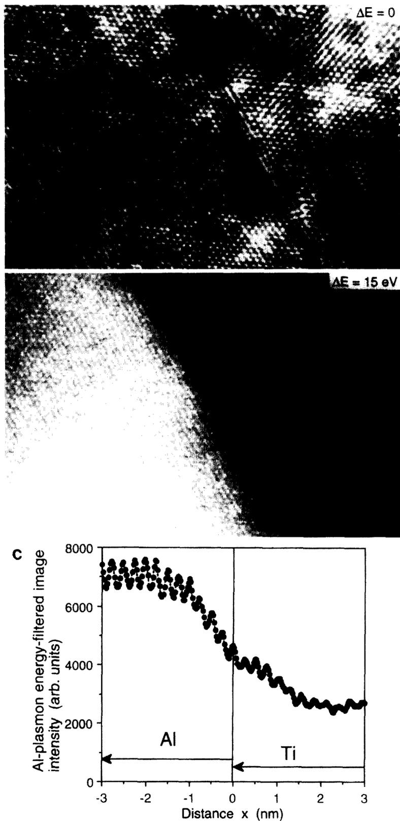
Fig. 7. (a) Zero-loss and (b) 15 eV Al-plasmon loss energy-selected HREM images of an edge-on Al/Ti (111) interface. Energy window  $\Delta = 4$  eV [10]. (c) An intensity line scan across the Al/Ti interface from the image recorded using the 15 eV Al-plasmon-loss electron image. This curve determines the spatial resolution of valence-loss electron imaging, provided the interface is atomically sharp and there is no interdiffusion.
