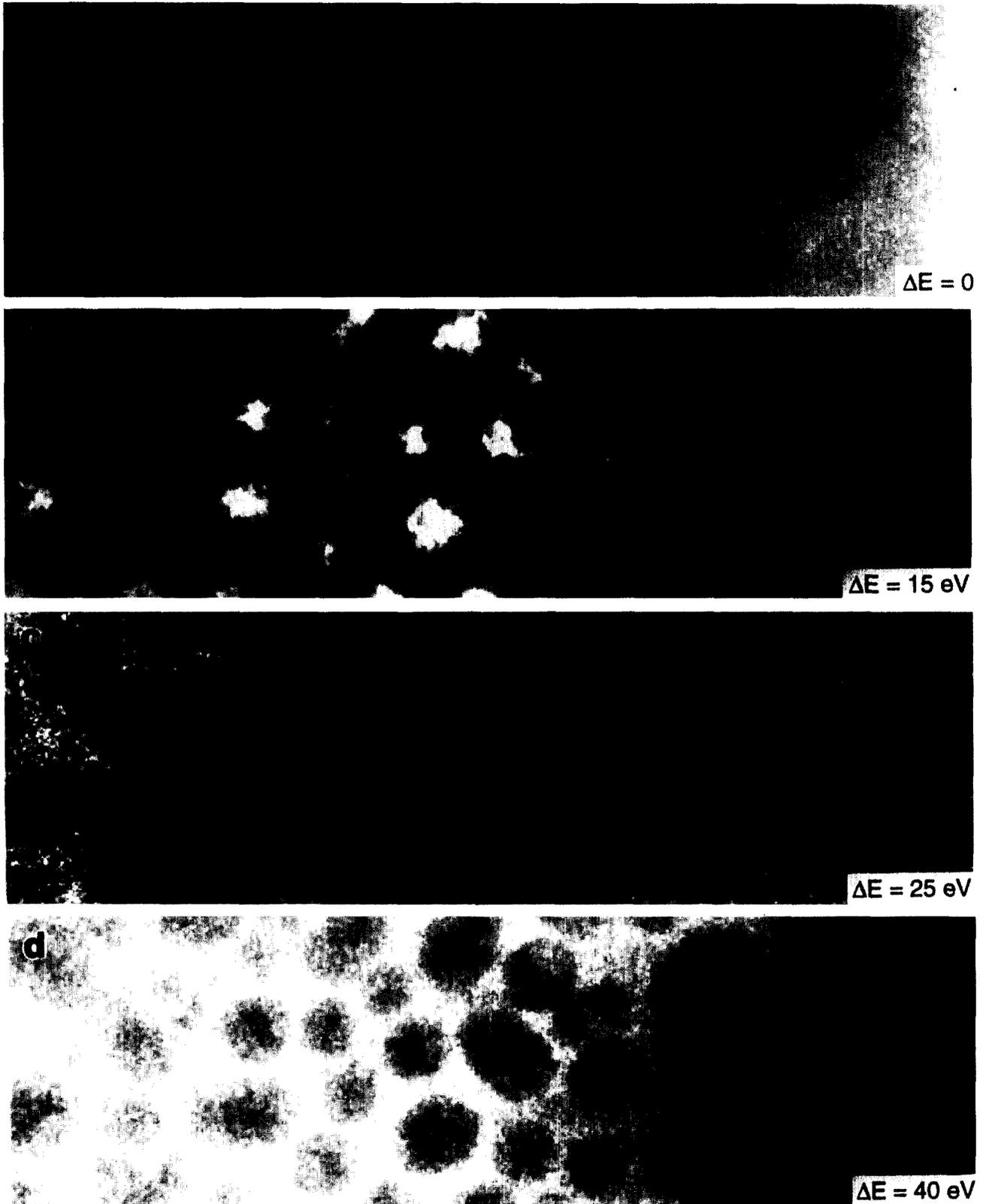
Fig. 2. (a) Zero-loss, (b) 15 eV plasmon-loss, (c) 25 eV plasmon-loss and (d) 40 eV peak energy-selected TEM images from the same specimen region of a 100 keV  $Y^+$  implanted alumina specimen. The energy selection window was centered at these energies specified and its width was 5 eV.
