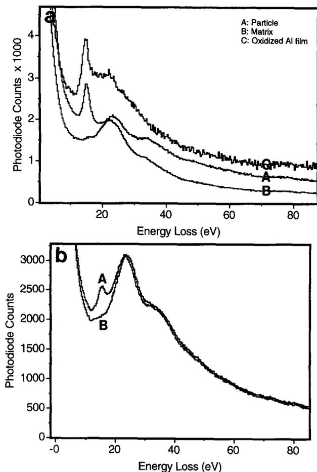
Fig. 4. Energy-loss spectra from (A) an embedded particle and (B) the adjacent amorphous matrix for (a) a large particle and (b) a small particle, where the spectrum C was acquired from a standard thin Al foil covered by alumina oxidation layers.
