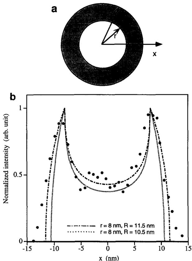
Fig. 8. (a) A spherical shell model of a compositionally porous Al particle, and (b) the projected atom density of the shell particle along the beam direction for two cases in comparison with the experimentally observed profile obtained from the particle B in Fig. 6(a).
