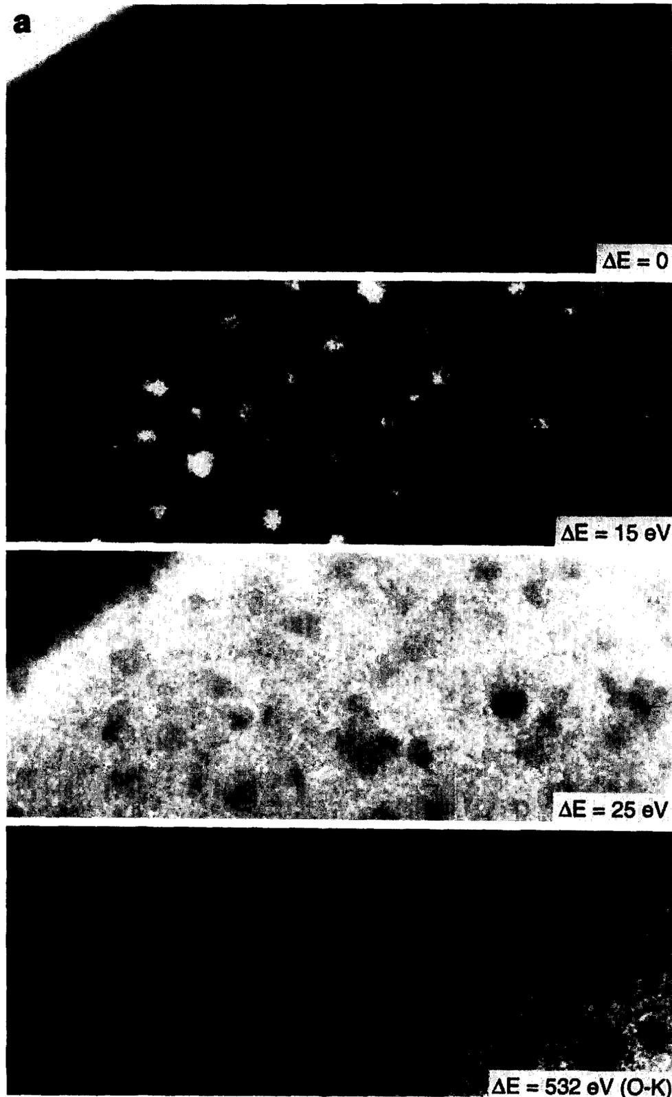
Fig. 3. (a) Zero-loss, (b) 15 eV plasmon-loss, (c) 25 eV plasmon-loss and (d) oxygen jump ratio energy-selected TEM images from the same specimen region of a 170 keV  $Y^+$  implanted alumina specimen. The energy selection window was centered at these energies specified and its width was 5 eV.
