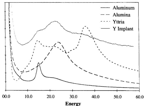
Fig. 1. A comparison of EELS spectra acquired from an aluminum foil, alumina, yttria and a yttrium implanted alumina sample for selecting the characteristic peaks which might be used for forming energy-filtered images. The implanted sample spectrum has been offset along the y-axis for clarity.
