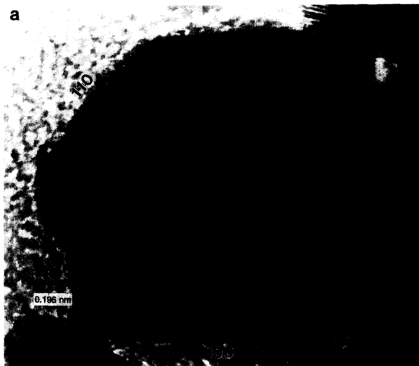
Fig. 4. HRTEM images of defected cubic-like Pt particles oriented along [001] , showing the formation of \{110\} facets.
