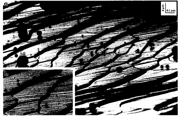
Fig. 5. (a) REM image of the \text{LaAlO}_3(110) surface, annealed at 1500°C for 20 h, showing the increase in the population of large surface terraces in comparison to those shown in Fig. 3. The arrowheads indicate possible {100} facets. (b) Enlargement of the image showing fine step-like contrast on surface terraces. Beam azimuth is near [001]. The image was recorded under the diffracting condition shown in Fig. 3b.
