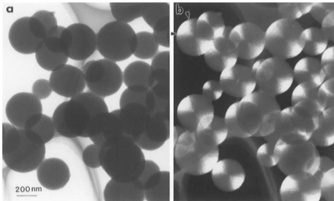
**Figure 2.** (a) Bright-field and (b) dark-field TEM images of the synthesized carbon spheres. The spheres are solid, clean, smooth, and without porosity. The dark-field image is recorded using part of the {101} reflection ring.
