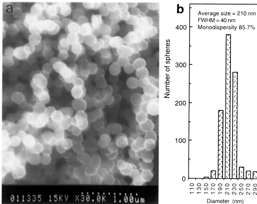
**Figure 1.** (a) SEM image of carbon spheres synthesized at 1100 °C, showing monodisperse size distribution as indicated by the plot in (b). The product is pure, and no carbon tubes or any other product was observed. The image was recorded at 15 kV using a Hitachi S800 SEM.
