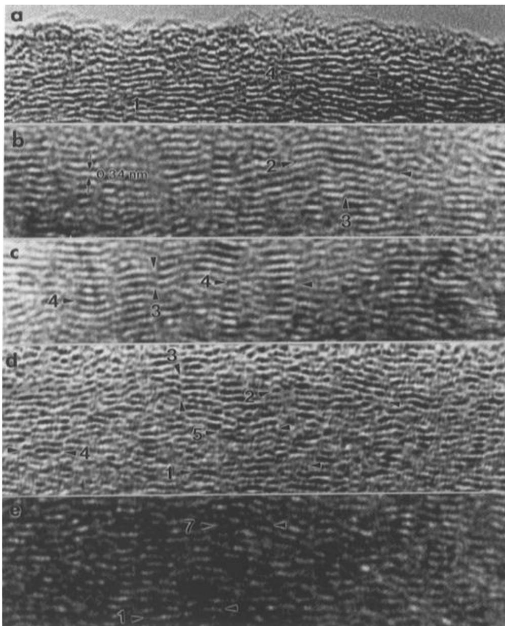
**Figure 6.** HRTEM images of the spherical carbon particles showing the various types of graphitic waving structures in the areas indicated by arrowheads. The sequence numbers appearing in the areas represent the structural models described in Figure 9. The interlayer distance is 0.34 nm in each image.
