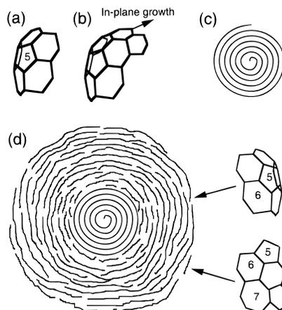
**Figure 8.** (a) Nucleation of a pentagon, (b) growth of a quasi-icosahedral shell, and (c) formation of a spiral shell carbon particle proposed by Kroto and McKay.<sup>7</sup> (d) Growth of a large size carbon sphere.
