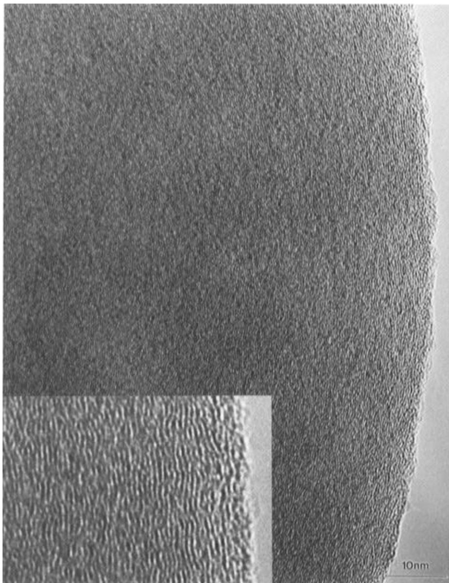
**Figure 3.** HRTEM image of a carbon sphere showing that the sphere is composed of a piling up of graphitic layers, with the *c*-axis approximately parallel to the radial direction. The inset is a magnified region.
