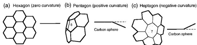
**Figure 7.** (a) Hexagonal, (b) pentagonal, and (c) heptagonal carbon ring structures in graphitic flakes. The curving of the graphitic flake resulting from these structures is schematically shown using the two-dimensional models for the convenience of HRTEM image interpretation, although the curving occurs on a 3-D surface.
