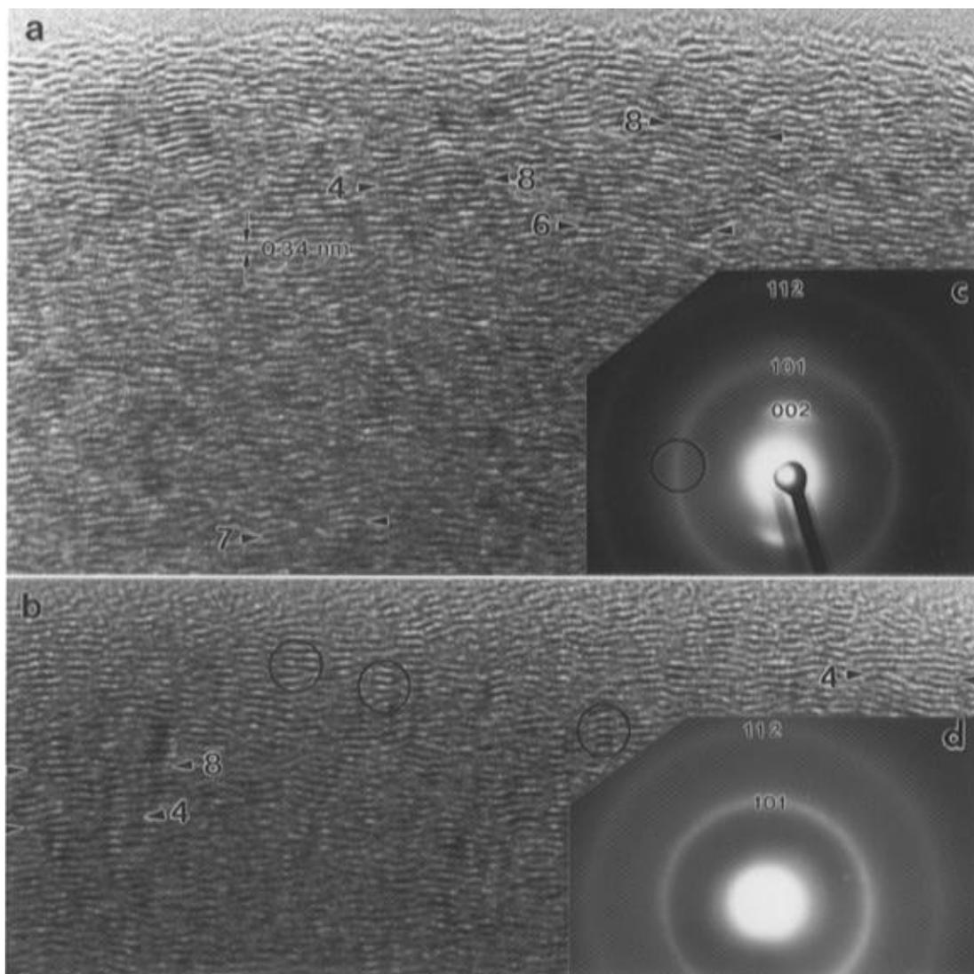
**Figure 5.** (a, b) HRTEM images of the spherical carbon particles near the edges, showing the graphitic waving structures. The sequence numbers appearing in the areas indicated by the paired arrowheads represent the structural models described in Figure 9. The interlayer distance is 0.34 nm. (c, d) Electron diffraction patterns recorded from a carbon sphere when the electron probe is positioned at the edge and the center of the sphere, respectively.
