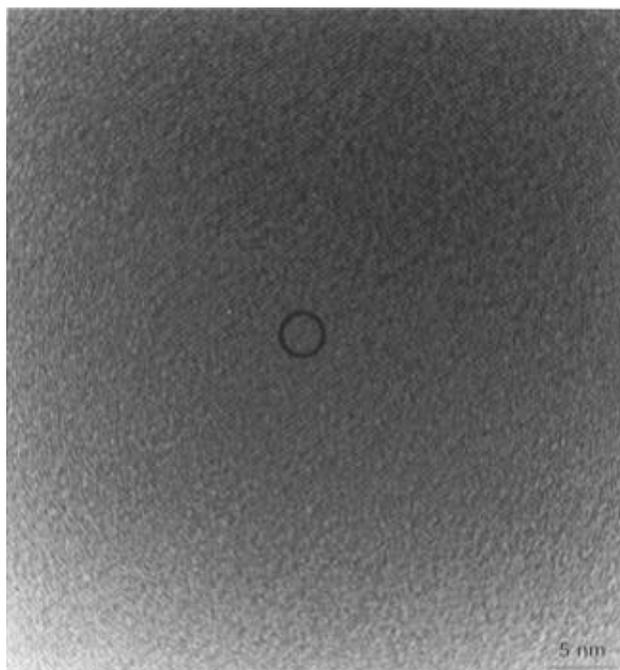
**Figure 4.** HRTEM image of a carbon sphere recorded near the center showing that the sphere is solid. The graphitic flakes around the center are imaged.
