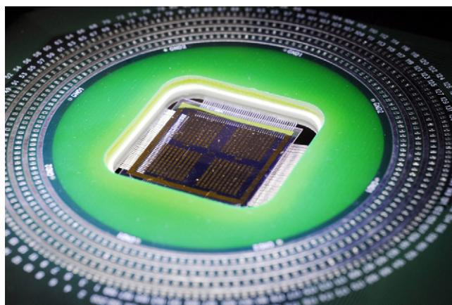
**Figure 1** An array of piezoelectrically modulated resistive memory (PRM) cells shown through an optical microscope. (Credit: Gary Meek, Georgia Tech.)
