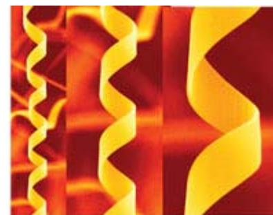
Scanning electron microscopy images of the semiconducting and piezoelectric zinc oxide nanohelix. (Courtesy: ZL Wang)
